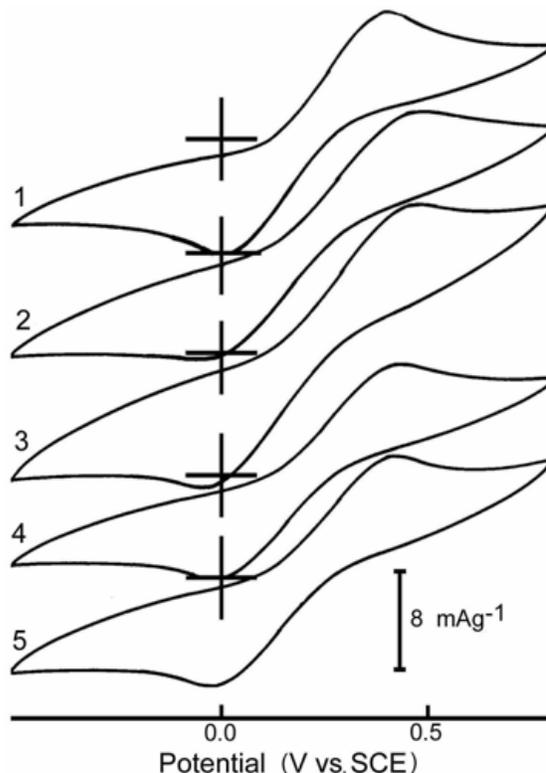
Figure (7) : Cyclic voltammograms of the [Fe(CN)<sub>6</sub>]<sup>4-</sup>/ [Fe(CN)<sub>6</sub>]<sup>3-</sup> couple on carbon electrodes (numbers as in table 1);  $\nu = 2$  mV/s.
