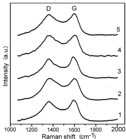
Figure (4) : Raman spectra of the combustion products (numbers as in table 2).
