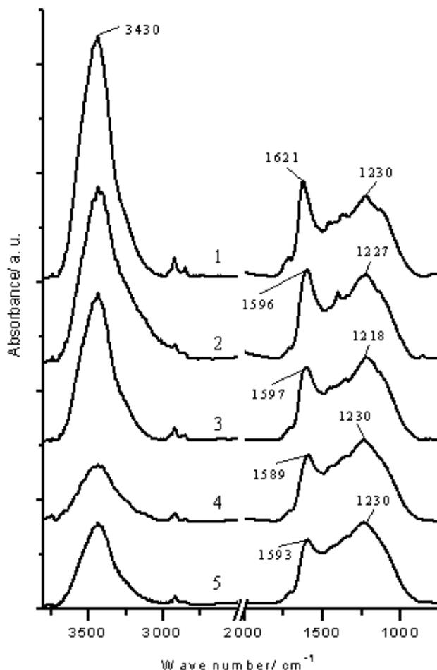
Figure (5) : FTIR transmittance spectra of the carbon materials (KBr pellets) (numbers as in Table 1).
