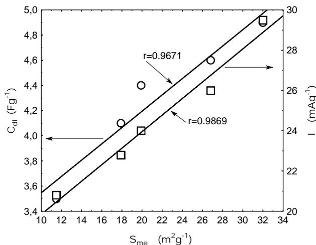
Figure (8) : Dependences of electrochemical capacity ( $C_{dl}$ ) and anodic peak current ( $I_{p,a}$ ) on the mesopore surface area of carbon electrode materials.
