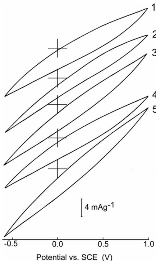
Figure (6) : Cyclic voltammograms of the carbon electrode materials (numbers as in table 1) recorded in a mixed electrolyte (75 ml aq. 0.1 M NaH<sub>2</sub>PO<sub>3</sub> and 25 ml ethanol) solution; sweep rate  $\nu = 1$  mV/s.
