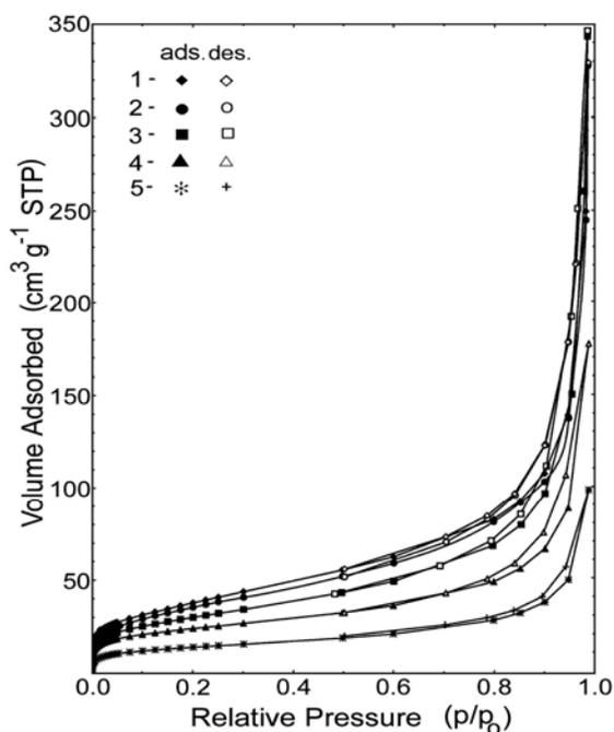
Figure (1) : Nitrogen adsorption-desorption isotherms at (77.4 K) of the combustion products: (1) C-C<sub>5</sub>Cl<sub>6</sub>, (2) C-CCl<sub>4</sub>, (3) C-C<sub>2</sub>Cl<sub>6</sub>, (4) C-C<sub>4</sub>Cl<sub>6</sub>, (5) C-C<sub>2</sub>Cl<sub>4</sub>.
