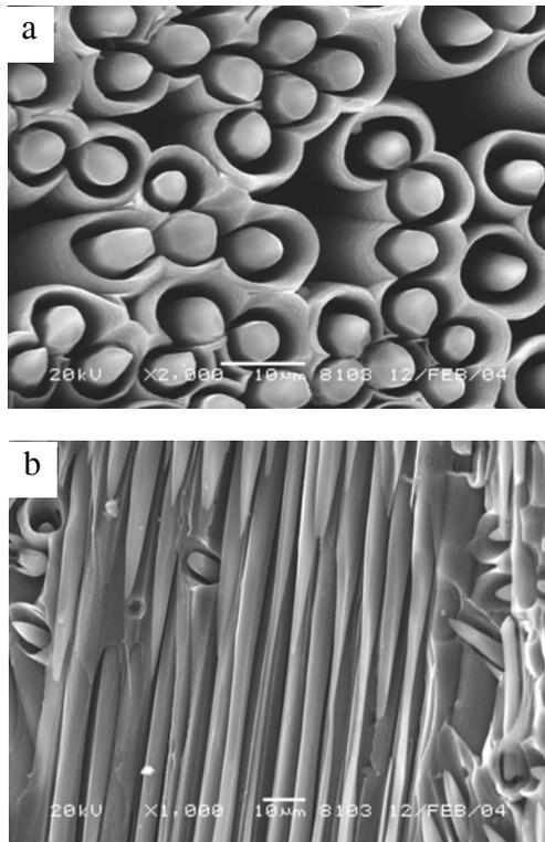
Figure (3) : Ablation morphologies of sample A.
