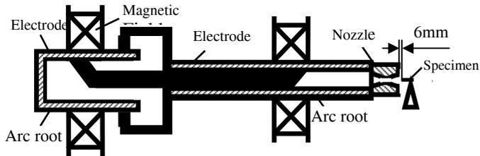
Figure (1) : Sketch of the arc heater
