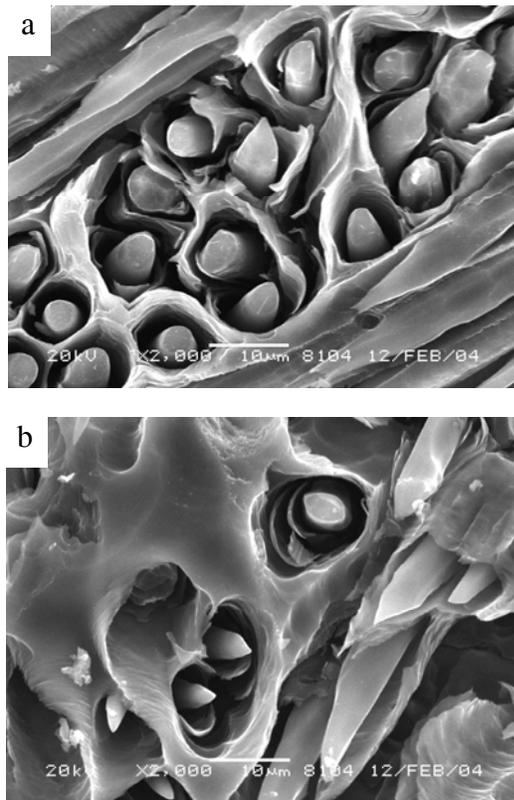
Figure (5) : Ablation morphologies of sample C.
