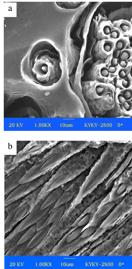
Figure (4) : Ablation morphologies of sample B.
