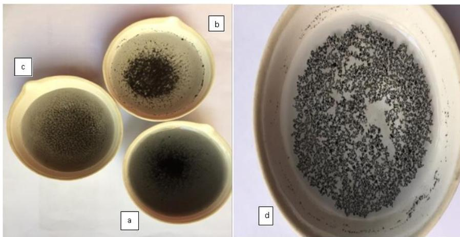
Figure (5): Simple water dispersibility test of a) burnt sample; b) PVA encapsulated as-synthesized sample; c) PVA encapsulated burnt sample; d) Dispersibility of as-synthesized sample in water.
