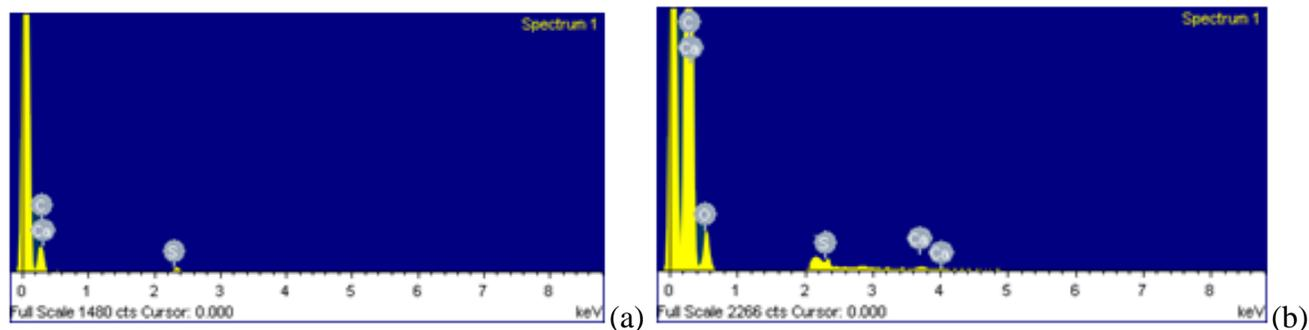
Figure (2): EDXA of a) as-synthesized sample and b) burnt sample.
