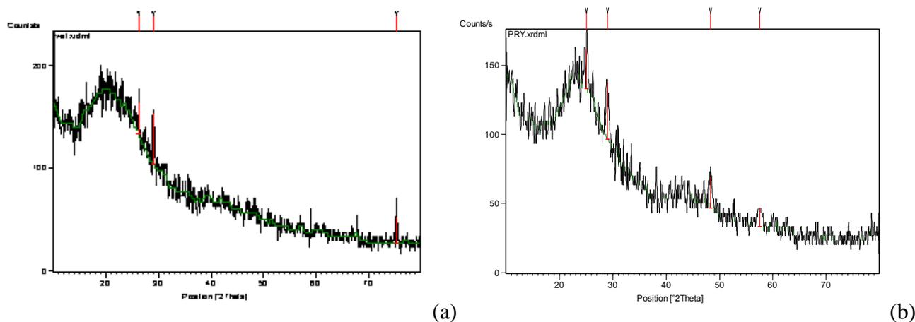
Figure (3): XRD of a) as-synthesized sample b) burnt sample.
