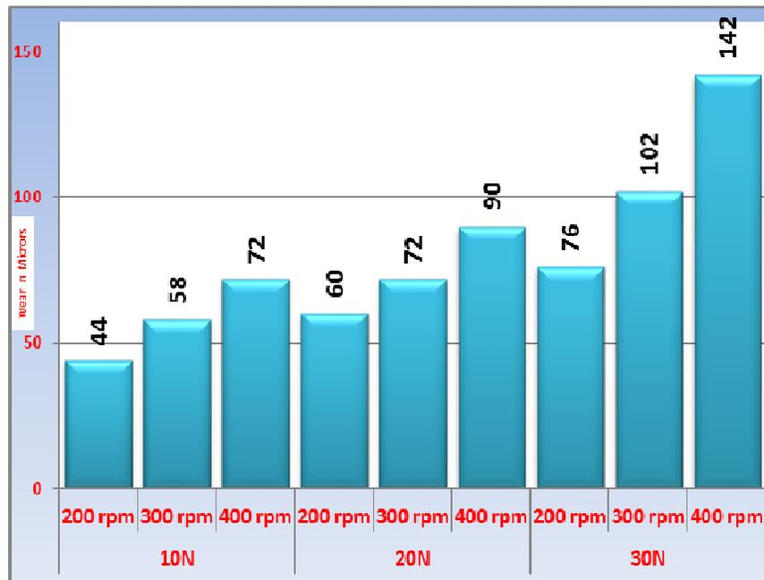
Figure (6): Effect of load and sliding speed and 220 mesh particle size on the wear loss of Al8011-SiC composites.
