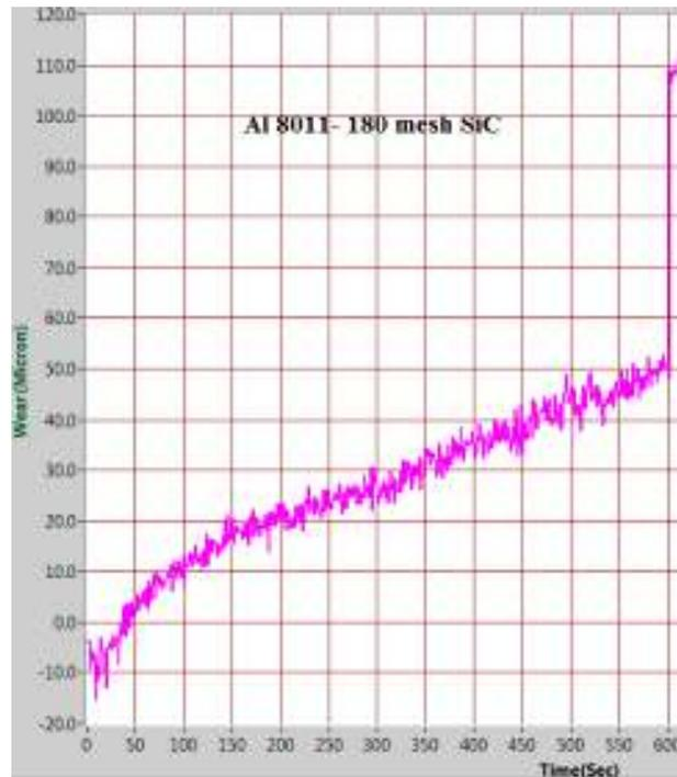
Figure (8): Typical wear curve of Al 8011-180 mesh SiC at a speed of 250 rpm, 15 N.
