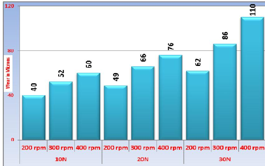
Figure (5): Effect of load and sliding speed and 180 mesh particle size on the wear loss of Al8011-SiC composites.
