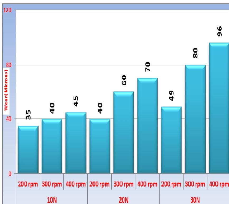
Figure (4): Effect of load and sliding speed and 150 mesh particle size on the wear loss of Al8011-SiC composites.
