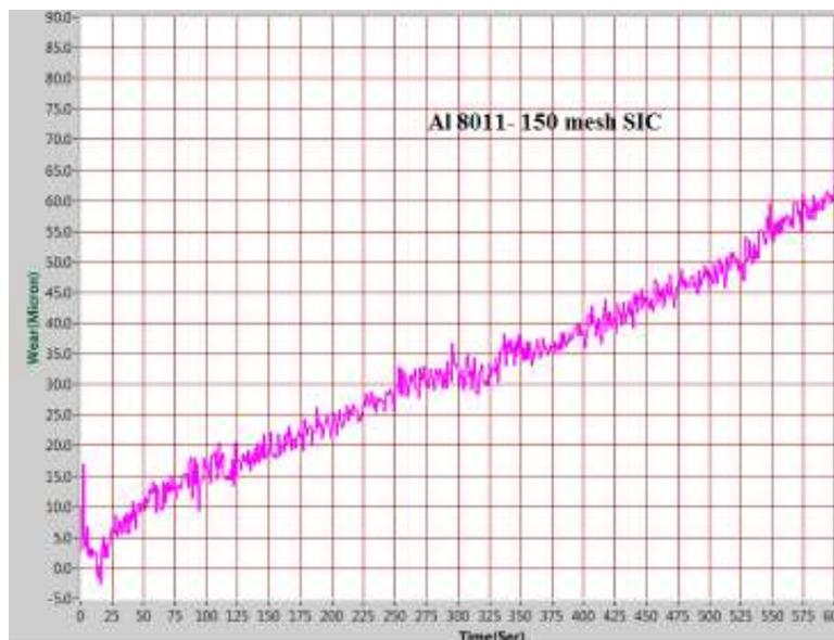
Figure (7): Typical wear curve of Al 8011-150 mesh SiC at a speed of 300 rpm, 25 N.
