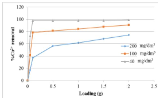
Figure (3): Effects of modified pineapple fiber waste carbon loading and total hardness on Ca<sup>2+</sup> removal.
