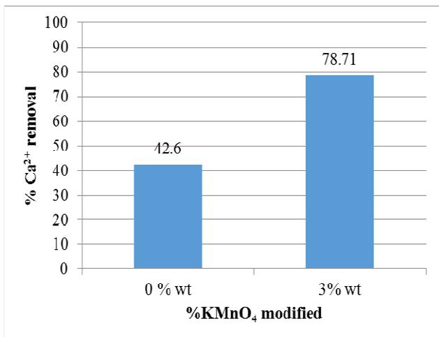
Figure (1): Comparison of Ca<sup>2+</sup> removal by unmodified and 3%wt KMnO<sub>4</sub> modified pineapple fiber waste carbon materials.
