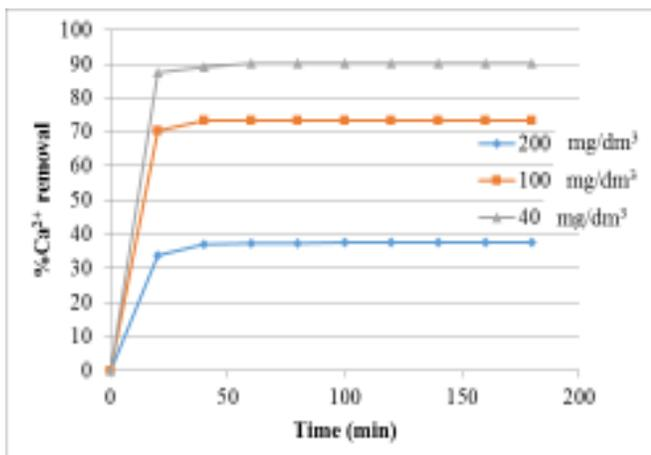
Figure (2): Effects of contact time and total hardness values on Ca<sup>2+</sup> removal efficiency.
