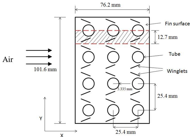
Figure (1): Top view of the computational domain
