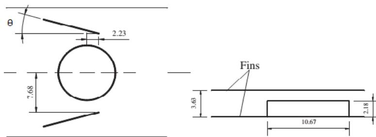
Figure (2): Placement of winglets near the tube wall
