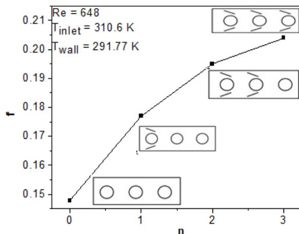
Figure (6c): friction losses with different number of rectangular winglet pairs
