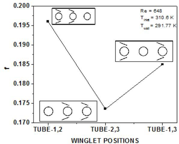
Figure (8b): variation of friction factor with different winglet positions
