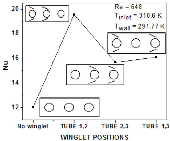
Figure (8a): variation of Nusselt number with different winglet positions
