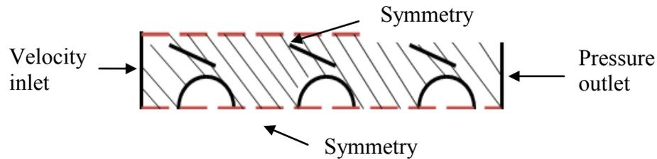
Figure (3): Boundary conditions from top view
