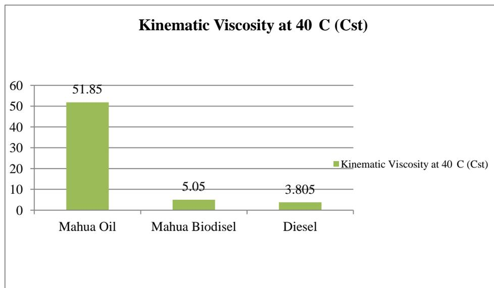
Graph 3: Kinematic Viscosity of Mahua oil, Mahua biodiesel and Diesel.
