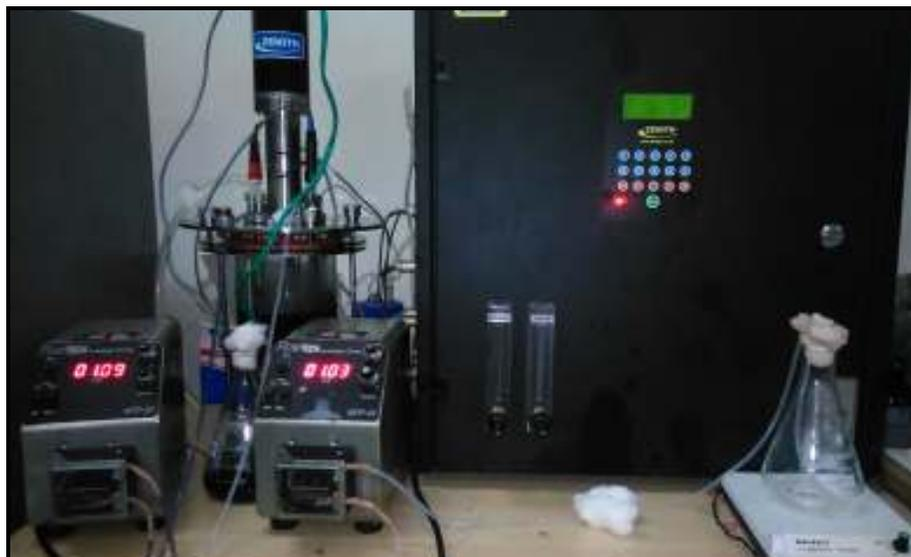
Figure (6): Continuous production of indigo in two phase bioreactor.
