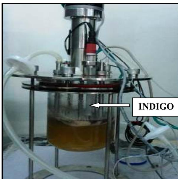
Figure (3): Bioreactor showing the production of indigo in the oil phase.
