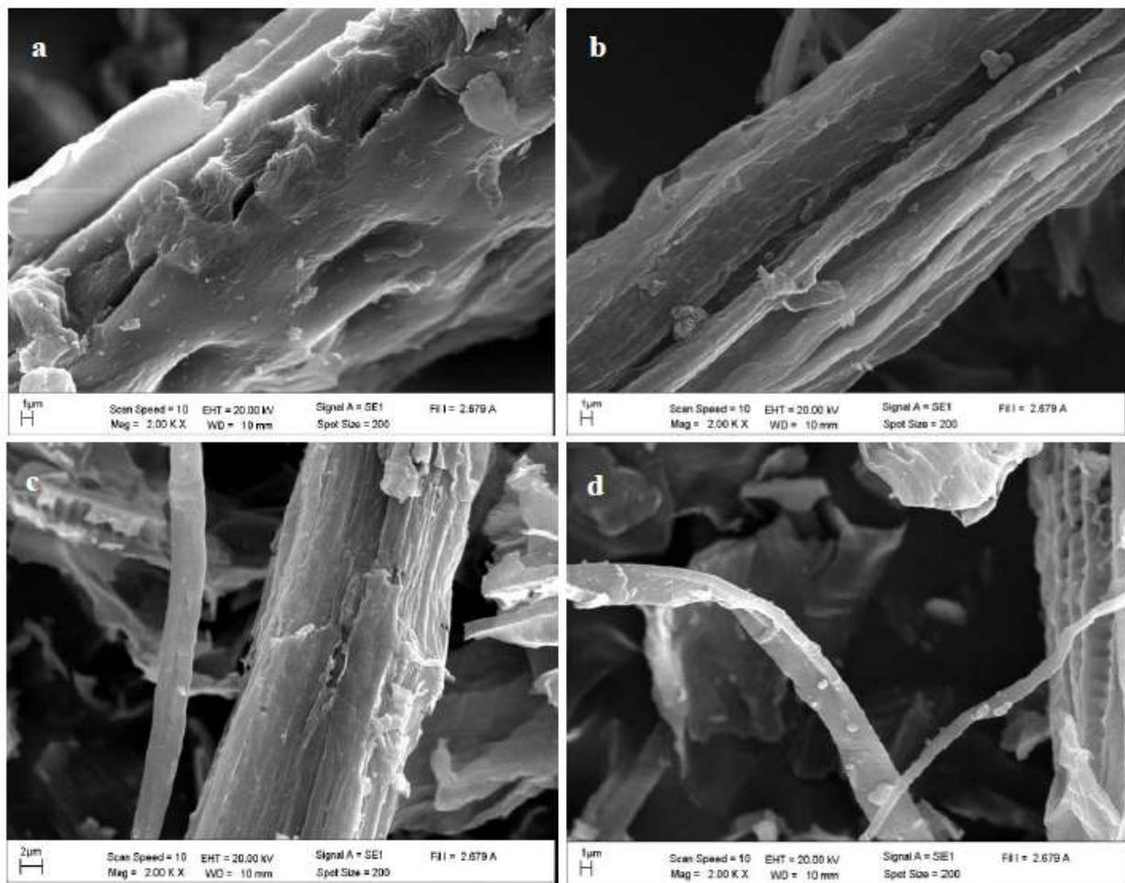
Figure (2): SEM micrographs of (a) FW (b) FWC at 500 °C (c) FWC at 600 °C (d) FWC at 700 °C.
