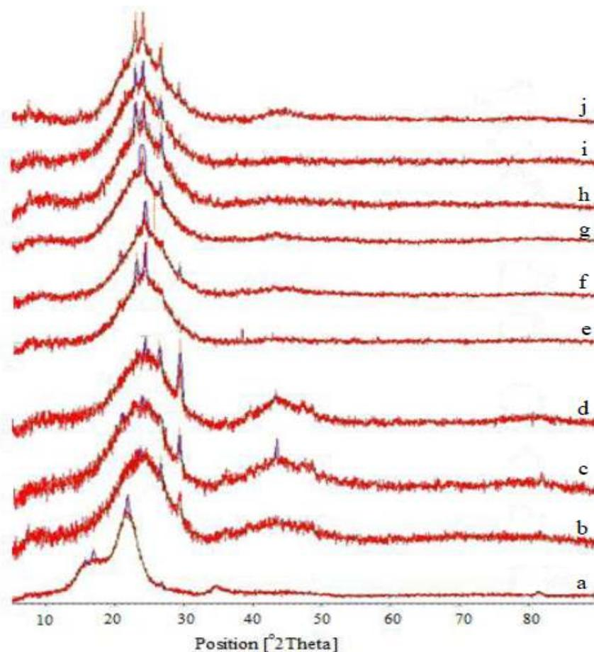
Figure (4): X-ray diffractograms of (a) FW (b) FWC at 500 °C (c) FWC at 600 °C (d) FWC at 700 °C (e) FWNPAC at 500 °C (f) FWNPAC at 600 °C (g) FWNPAC at 700 °C (h) FWPAC at 500 °C (i) FWPAC at 600 °C (j) FWPAC at 700 °C.
