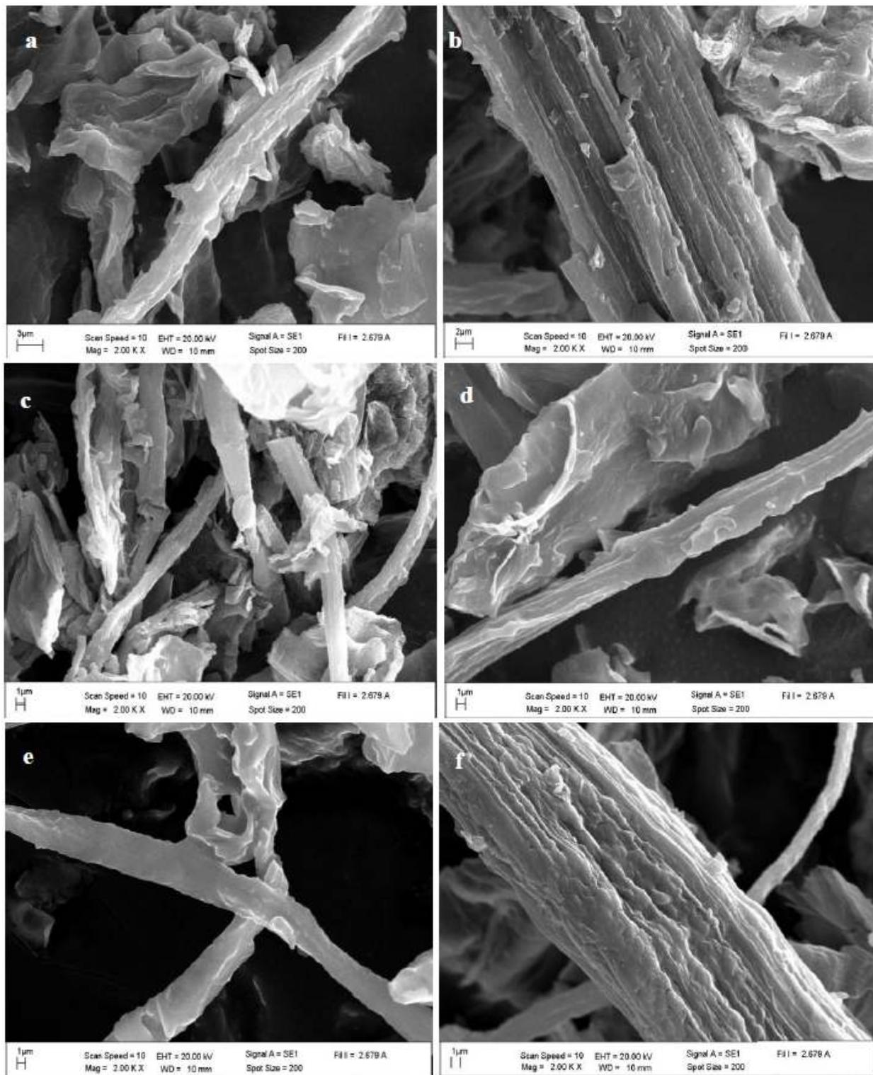
Figure (3): SEM micrographs of (a) FWNPAC at 500 °C (b) FWNPAC at 600 °C (c) FWNPAC at 700 °C (d) FWPAC at 500 °C (e) FWPAC at 600 °C (f) FWPAC at 700 °C.
