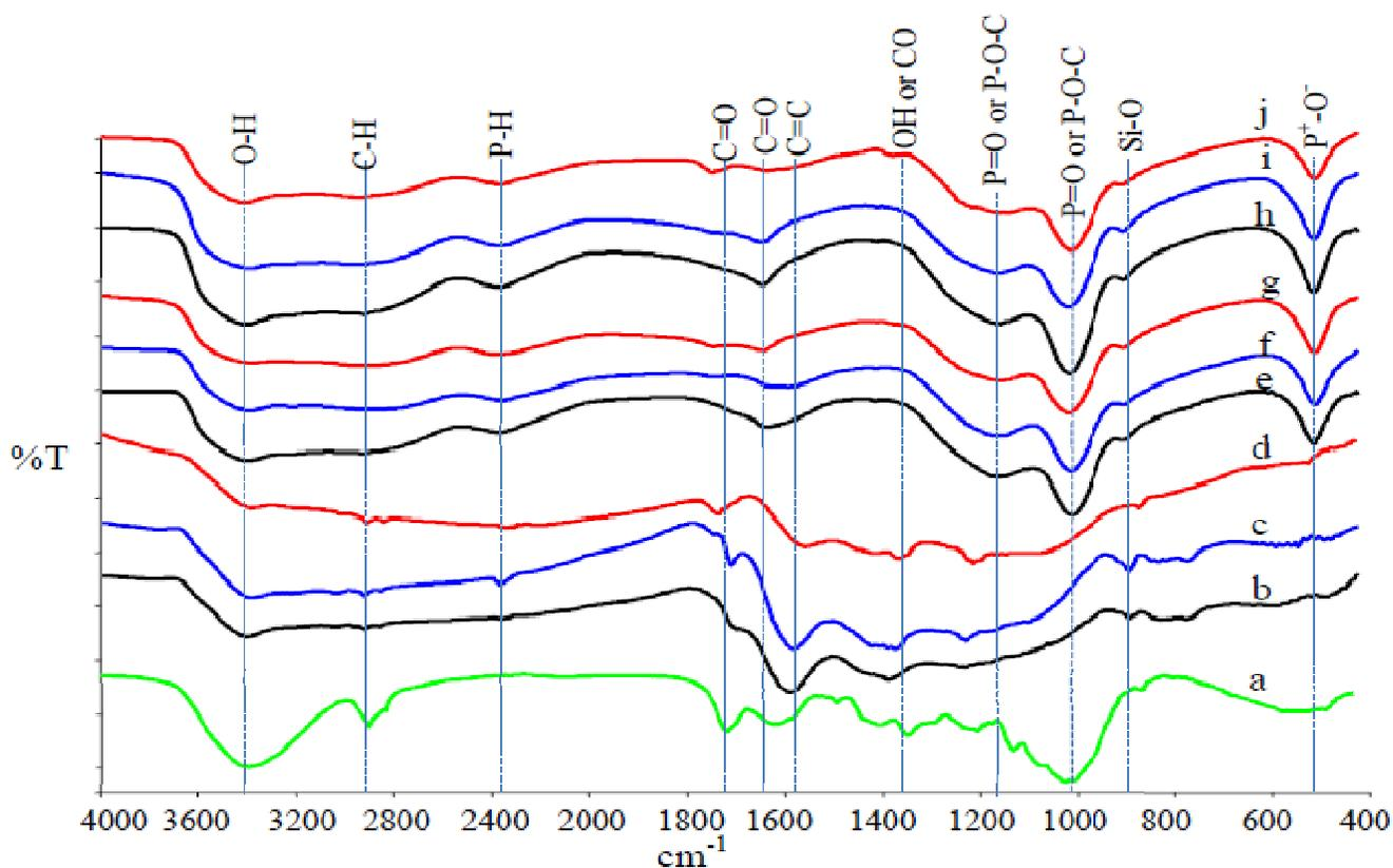
Figure (1) FTIR spectra of (a) FW (b) FWC at  $500\text{ }^{\circ}\text{C}$  (c) FWC at  $600\text{ }^{\circ}\text{C}$  (d) FWC at  $700\text{ }^{\circ}\text{C}$  (e) FWN PAC at  $500\text{ }^{\circ}\text{C}$  (f) FWN PAC at  $600\text{ }^{\circ}\text{C}$  (g) FWN PAC at  $700\text{ }^{\circ}\text{C}$  (h) FWPAC at  $500\text{ }^{\circ}\text{C}$  (i) FWPAC at  $600\text{ }^{\circ}\text{C}$  (j) FWPAC at  $700\text{ }^{\circ}\text{C}$ .
