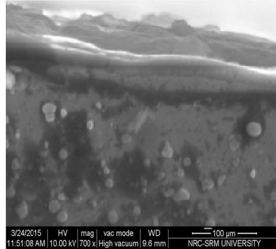
Figure (1) : SEM micrograph of cross-section of worn TiCN coated die segment.
