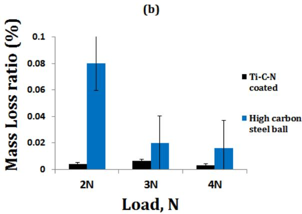
Figure (6b): Total wear of High carbon steel ball and Ti-C-N coated at different loads.
