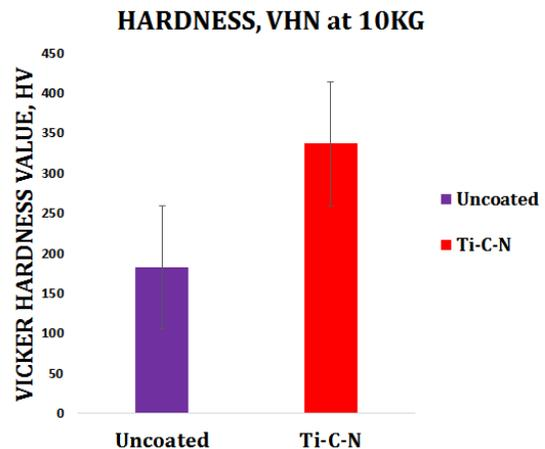
Figure (4): Micro-hardness of the coated specimen.
