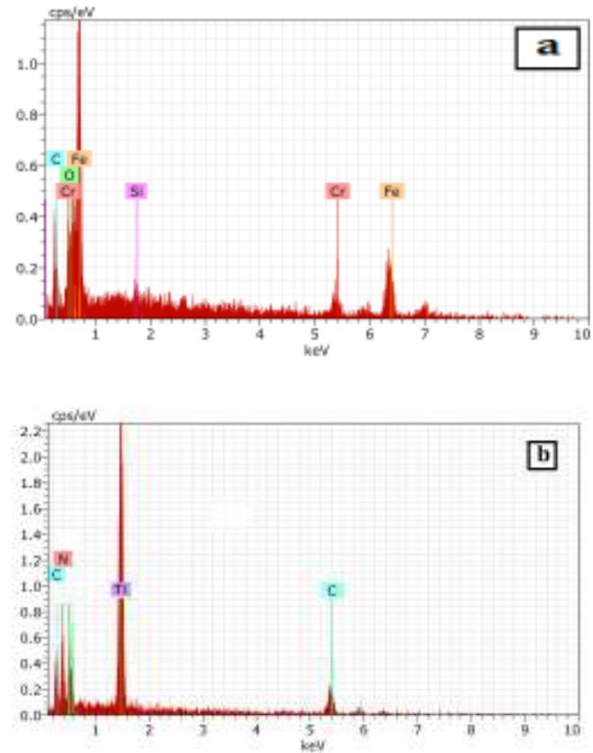
Figure (2): EDS analyses for worn surfaces of a) Uncoated substrate and b) Ti-C-N coated substrate.
