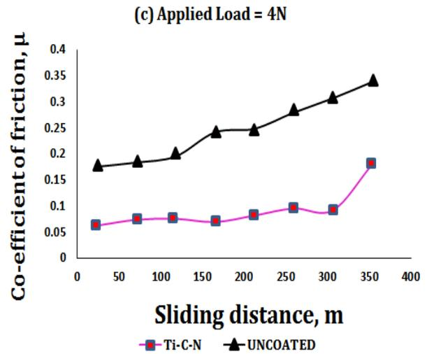
Figure (5): The co-efficient of friction of uncoated and coated films at different applied loads : (a) applied load = 2N, (b) applied load = 3N and (c) applied load = 4N.
