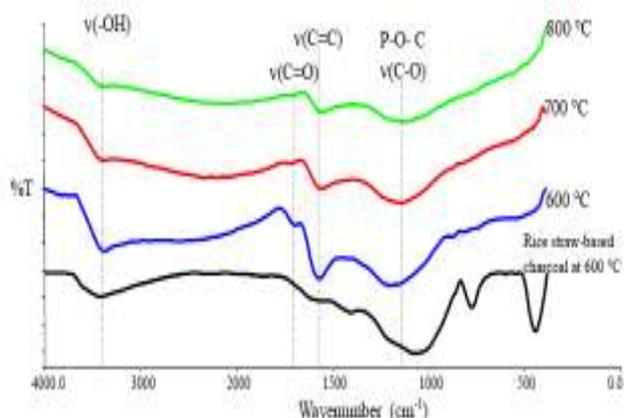
Figure (2): FTIR spectra of rice straw based activated carbons pyrolyzed between  $600\text{ }^{\circ}\text{C}$  and  $800\text{ }^{\circ}\text{C}$ .
