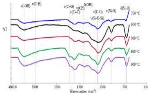
Figure (1): FTIR spectra of rice straw based charcoals carbonized between  $300\text{ }^{\circ}\text{C}$  and  $700\text{ }^{\circ}\text{C}$ .
