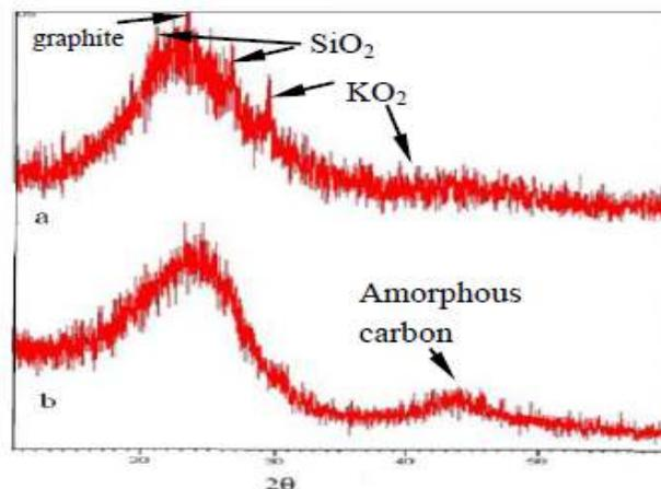
Figure (4): X-ray diffractograms of rice straw based charcoal carbonized at 600 °C (a) and rice straw based activated carbon activated at 800 °C (b).
