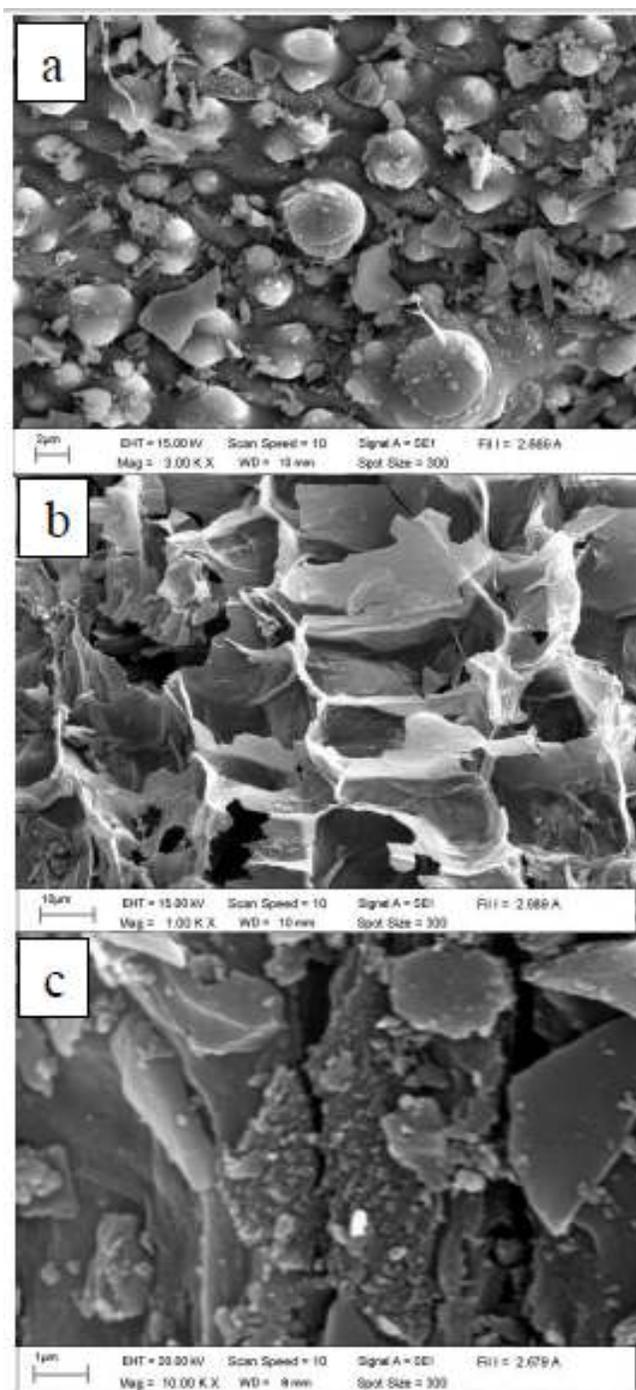
Figure (3): Scanning electron micrographs of rice straw base charcoal carbonized at 600 °C (a), rice straw based activated carbon activated at 800 °C, mag. 1000 X (b), and rice straw based activated carbon activated at 800 °C, mag. 10000 X (c)
