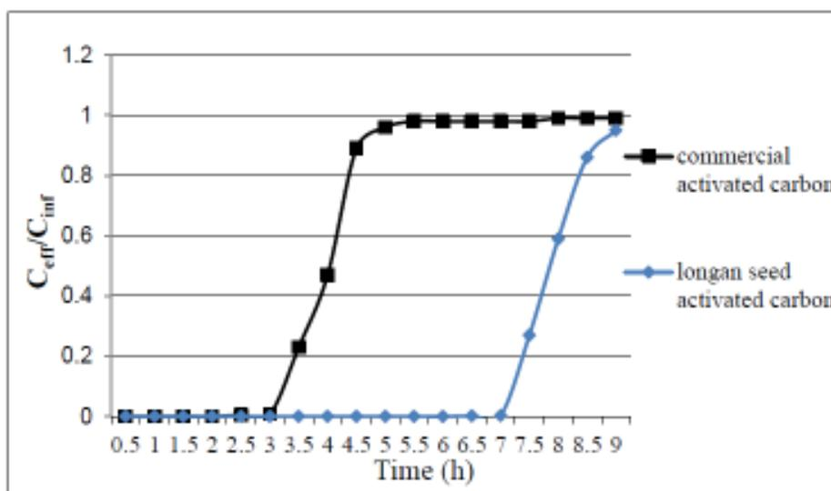
Figure (2): The breakthrough curves for pH 7 and 40 ppm lead solution passed through activated carbons.
