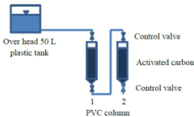
Figure (1): The schematic diagram of fixed-bed double column set up used in this work.
