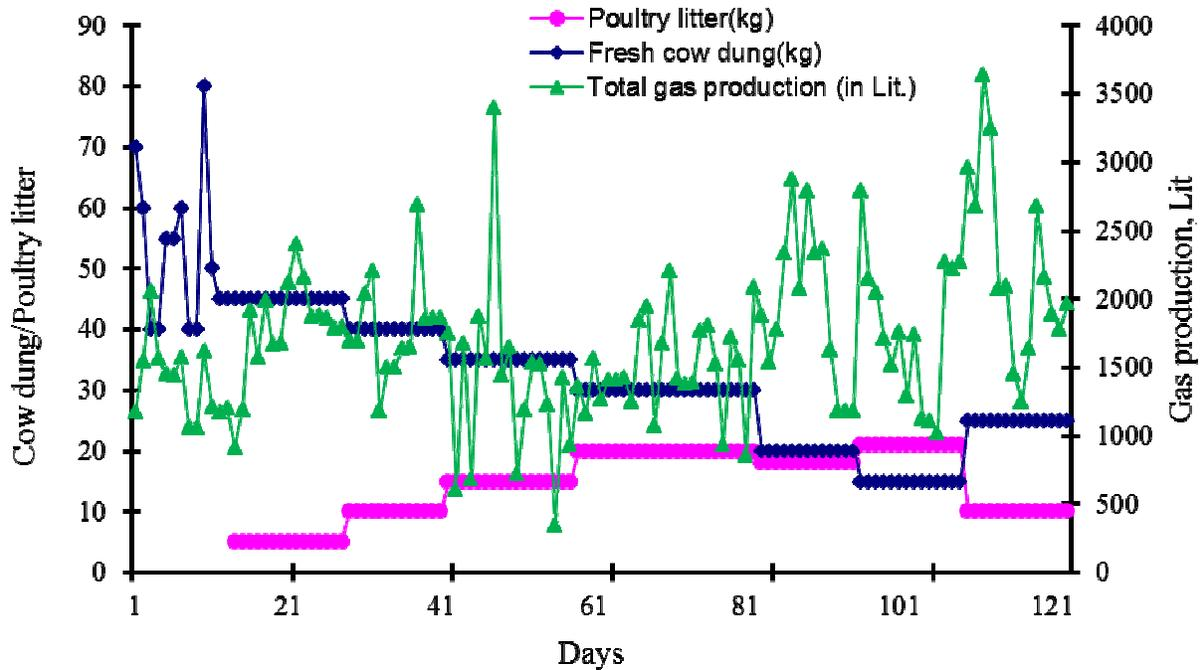
Figure (3): Daily gas production in response to feed stock substitution of cowdung with BFL.
