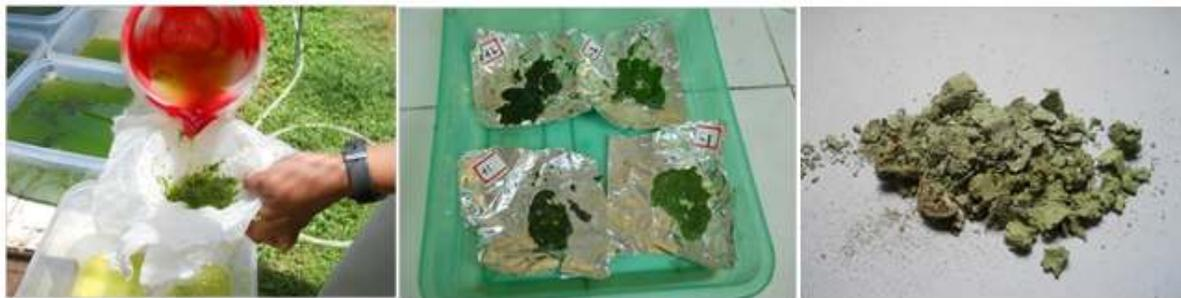
Figure (2, left): Harvesting of algae using a 50  $\mu$  nylon mesh.
