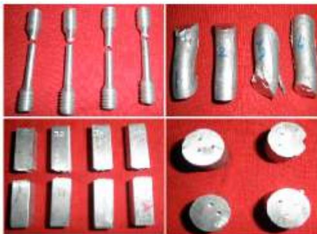
Figure (5): Tensile and Compression Tested Specimens
