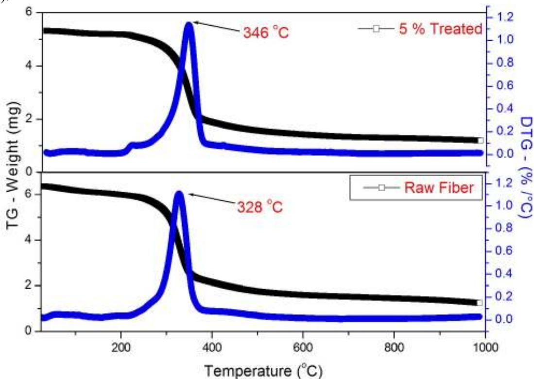
Figure (2): TGA/DTG analysis of raw fibre and 5% NaOH treated fibre.
