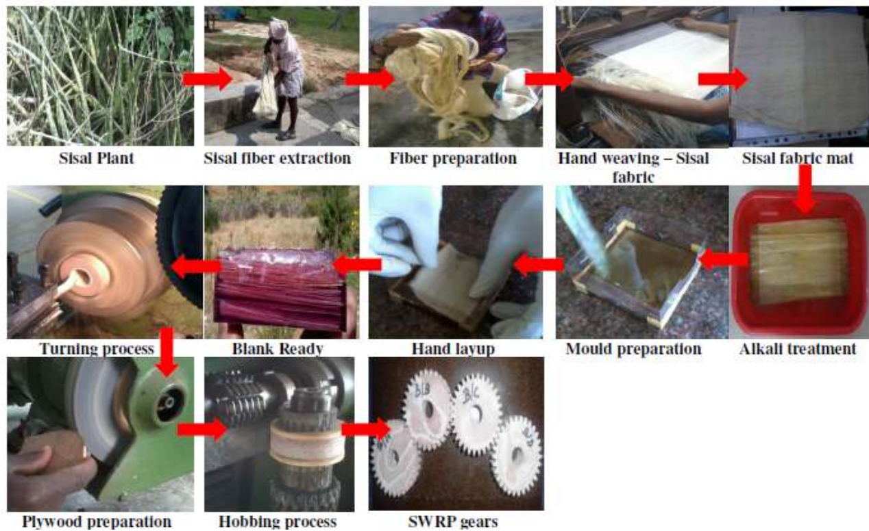
Figure (1): Preparation of SWRP gears through hand layup process.
