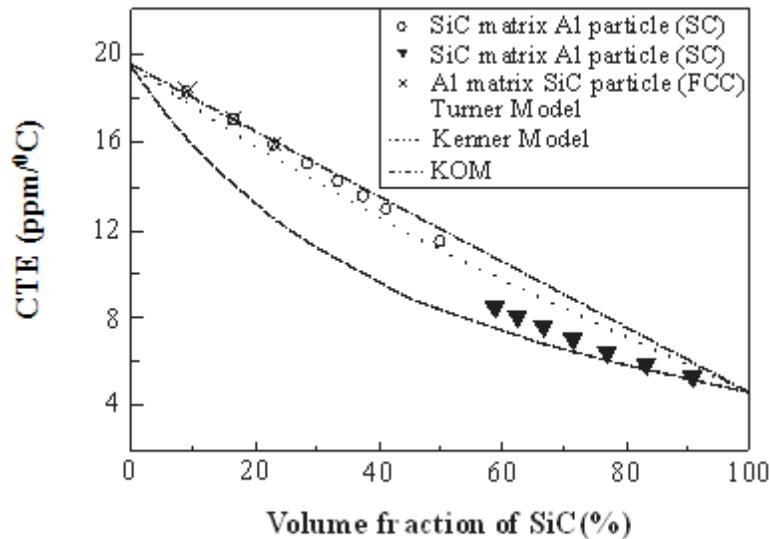
Figure (5): Calculated CTEs of MMC for simple cubic site SiC, simple cubic site Al, and face centered cubic site SiC
