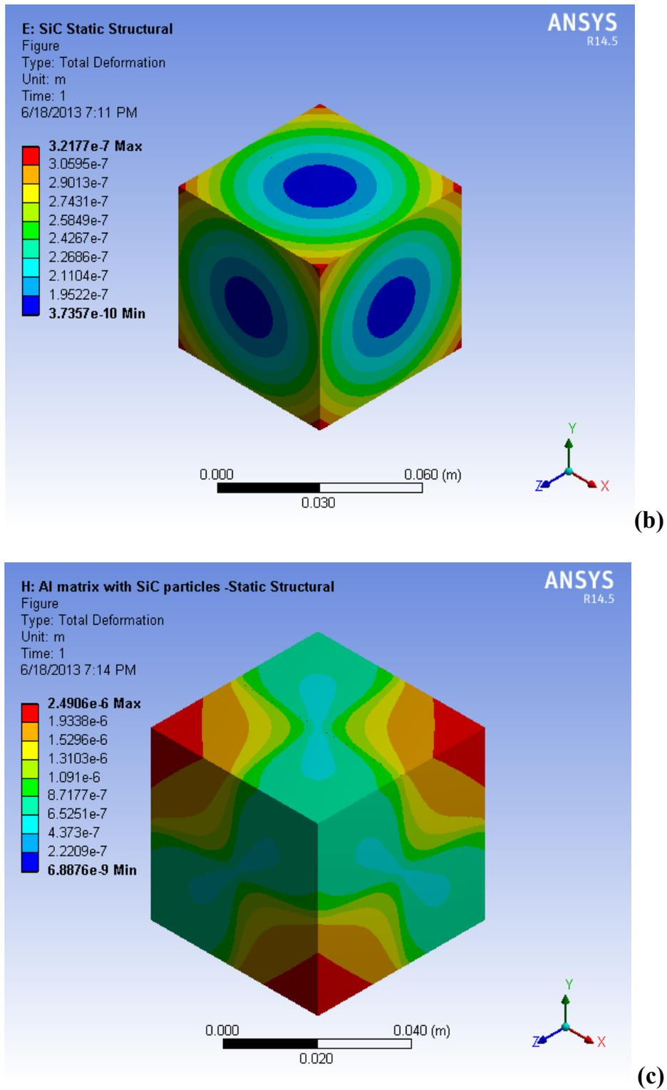
Figure (8): (a-c) Total deformations in Al-SiC Material
