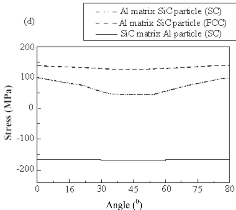
Figure (7): The principal stress for Al through the path.
