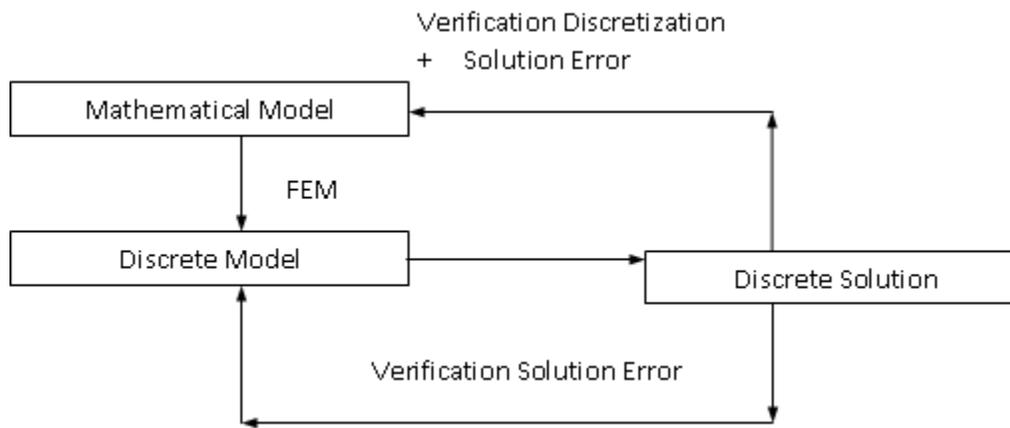
Figure (1): Finite Element Procedures
