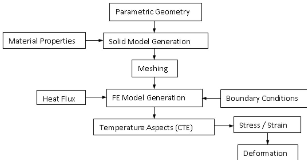
Figure (2): Procedure for finite element analysis
