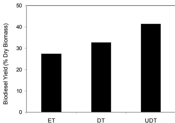
Figure (2) : Biodiesel Yield in various processes (ET – Extraction and Transesterification; DT – Direct Transesterification; UDT – Ultrasound assisted Direct Transesterification)
