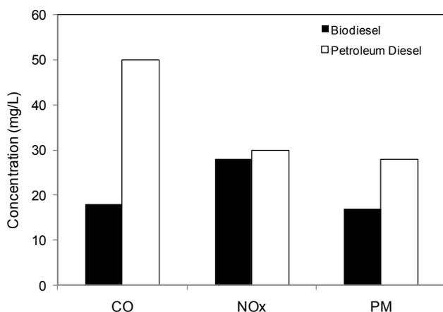
Figure (3) : Emission comparison between Biodiesel and Petroleum Diesel
