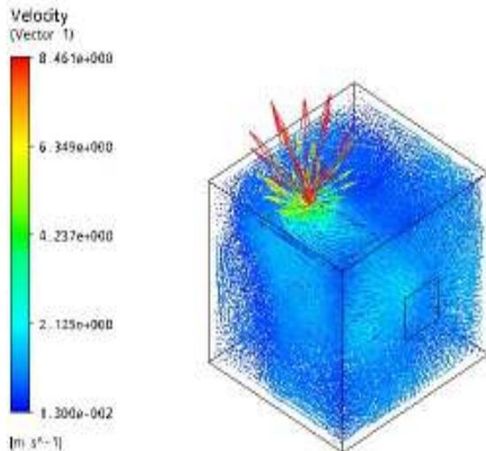
Figure (15): Velocity Streamline for natural ventilation system (100W heating).
