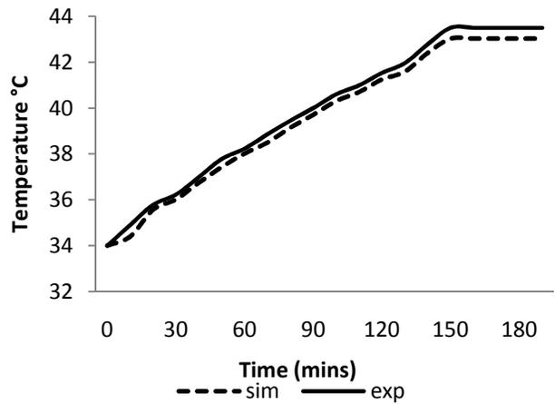
Figure (9a): Experimental and numerical Temperature variation for 50 W at selected RTD location with natural ventilation at Location 1.
