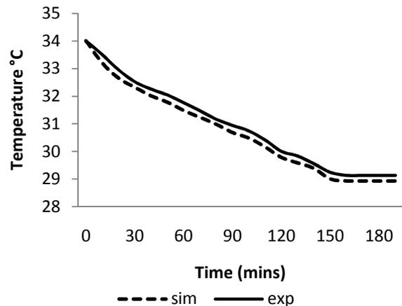
Figure (12a): Experimental and numerical Temperature variation for 50W at the selected RTD location with induced natural ventilation at Location 1.
