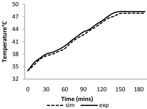
Figure (10b): Experimental and numerical Temperature variation for 100W at selected RTD location with natural ventilation at Location 2.
