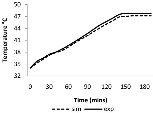
Figure (10a): Experimental and numerical Temperature variation for 100W at selected RTD location with natural ventilation at Location 1.
