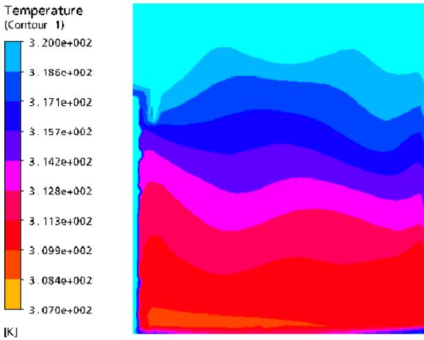
Figure (7): Temperature contour for natural ventilation system (100W heating).
