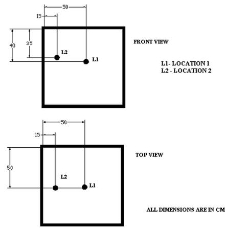
Figure (3): Location for selected RTDs for simulation
