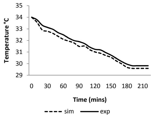
Figure (14a): Experimental and numerical Temperature variation for 150W at the selected RTD location with induced natural ventilation at Location 1.
