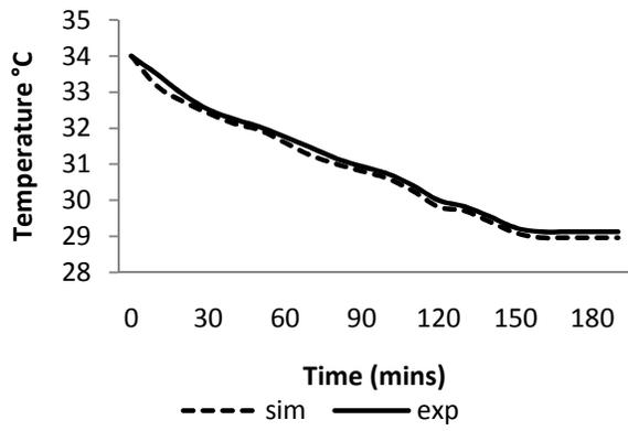
Figure (12b): Experimental and numerical Temperature variation for 50W at the selected RTD location with induced natural ventilation at Location 2.
