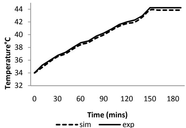
Figure (9b): Experimental and numerical Temperature variation for 50W at selected RTD location with natural ventilation at Location 2.
