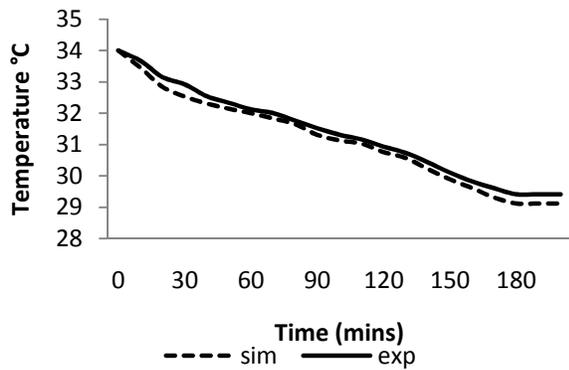
Figure (13a): Experimental and numerical Temperature variation for 100W at the selected RTD location with induced natural ventilation at Location 1.
