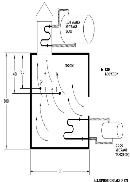
Figure (1): Concept of augmented natural ventilation using hot and cool sources
