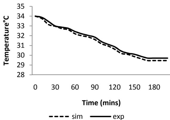
Figure (13b): Experimental and numerical Temperature variation for 100W at the selected RTD location with induced natural ventilation at Location 2.
