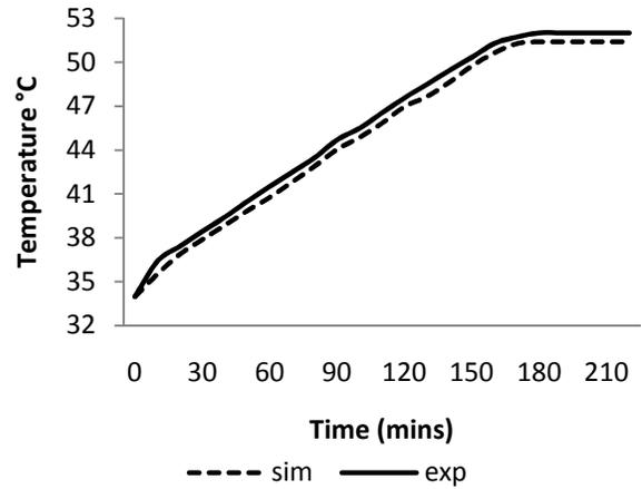
Figure (11b): Experimental and numerical Temperature variation for 150W at selected RTD location with natural ventilation at Location 2.
