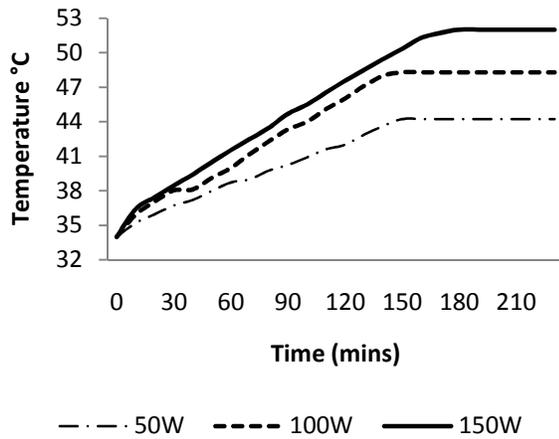
Figure (5b): Experimental Temperature variation at the selected RTD location with natural ventilation at Location 2.
