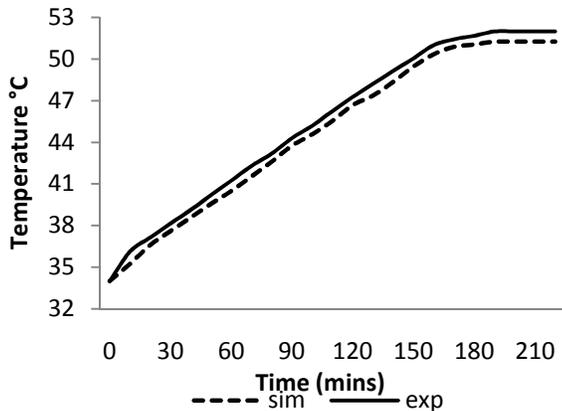
Figure (11a): Experimental and numerical Temperature variation for 150W at selected RTD location with natural ventilation at Location 1.
