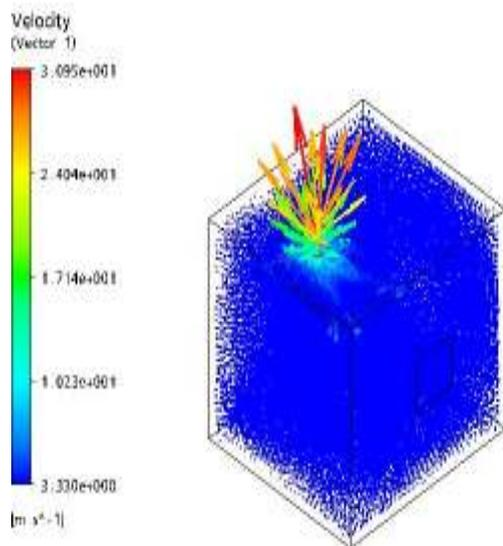
Figure (16): Velocity Streamline for induced natural ventilation system (100W heating).
