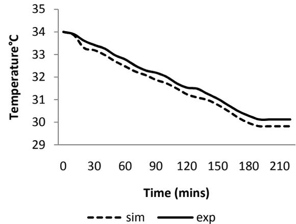
Figure (14b): Experimental and numerical Temperature variation for 150W at the selected RTD location with induced natural ventilation at Location 2.
