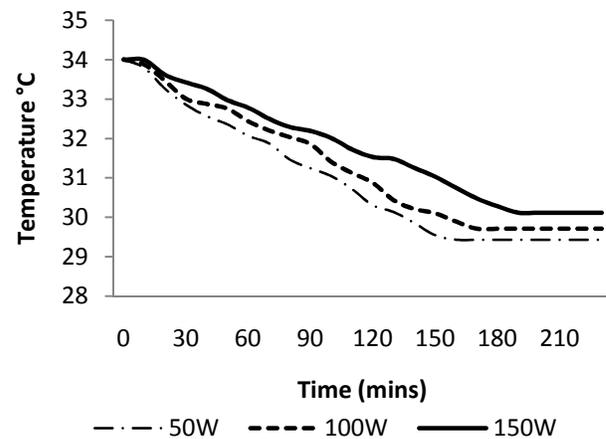
Figure (6b): Experimental Temperature variation at the selected RTD location with induced natural ventilation at Location 2.
