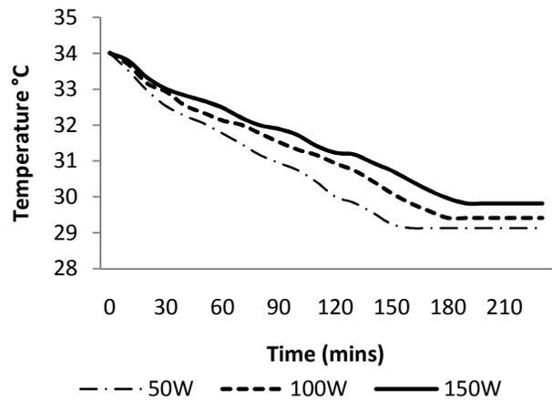
Figure (6a): Experimental Temperature variation at the selected RTD location with induced natural ventilation at Location 1.
