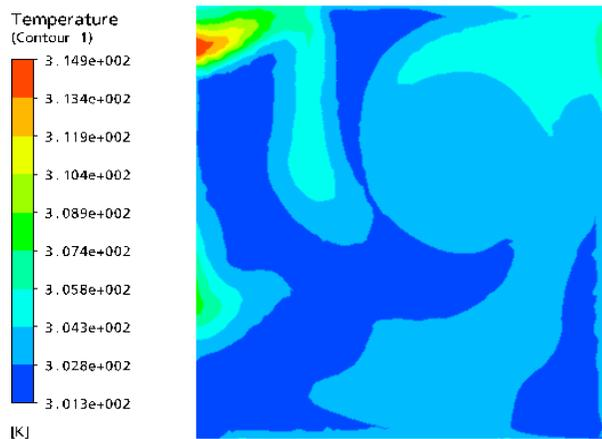
Figure (8): Temperature contour for induced natural ventilation system (100W heating).
