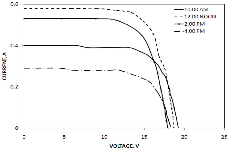
**Figure (3): I-V Characteristics of PV panel without reflector on the optimum day with panel in horizontal position**
