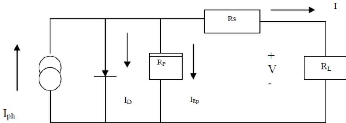
**Figure 1: Equivalent circuit of a PV cell**
