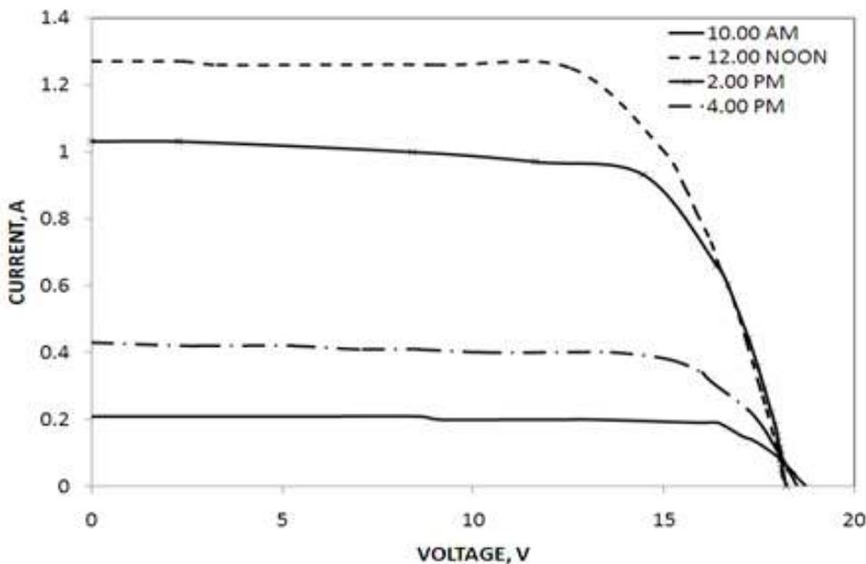
**Figure (4): I-V Characteristics of PV panel with reflector on the optimum day with panel at 30° inclination**
