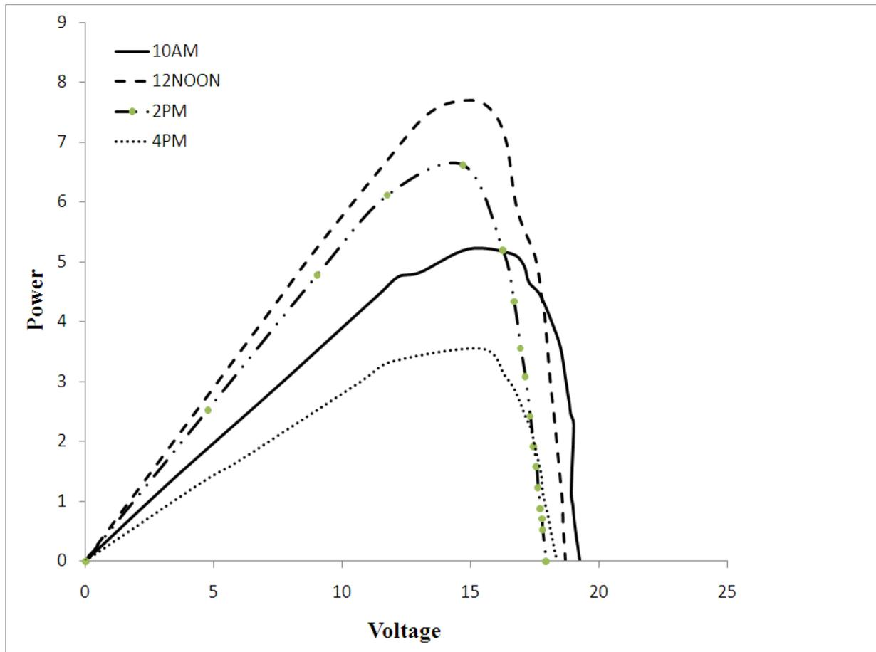
**Figure (5) : Power v/s voltage without reflector on the optimum day under case1 condition**
