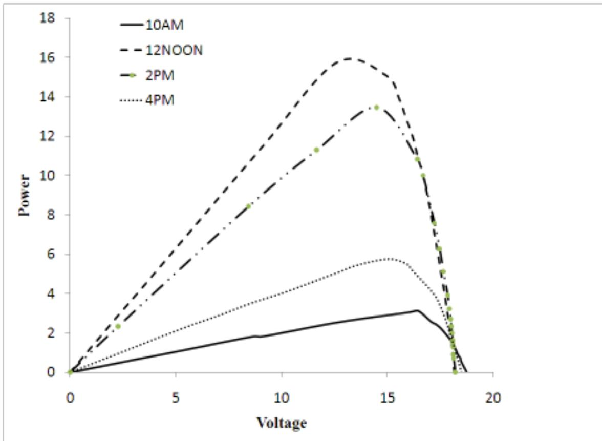
**Figure (6): Power v/s voltage with reflector on the optimum day under Case IV condition**
