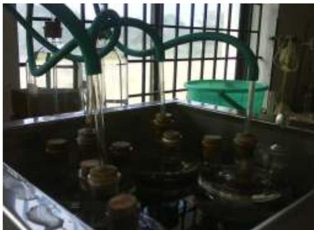
Figure (2) : The reactor set up in thermostat.
