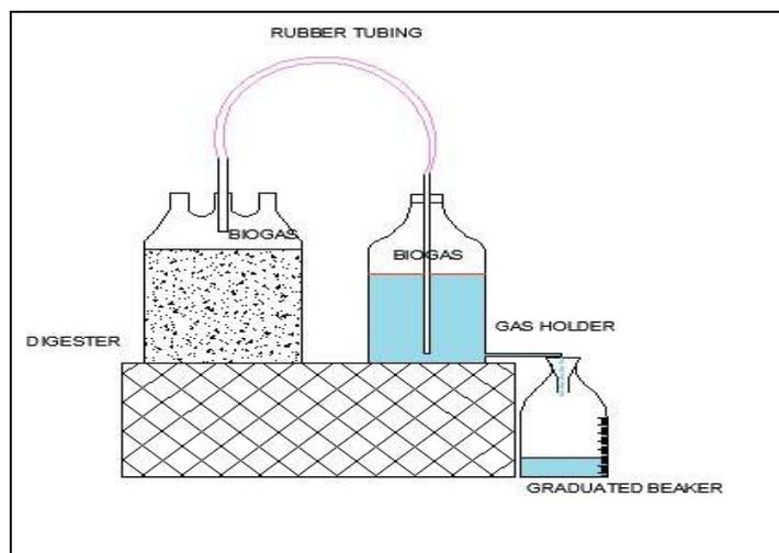
Figure (1) : Schematic representation of semi-continuous reactor.
