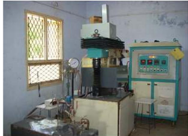
Figure (3) : ECM set up for non - rotating tool experiment.
