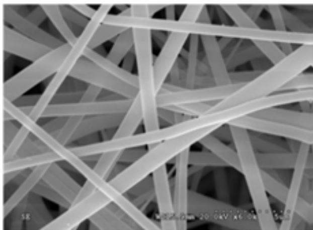
Figure (7) : Setup 1: 15 kV and 70 mm : 669 nm average fiber diameter
