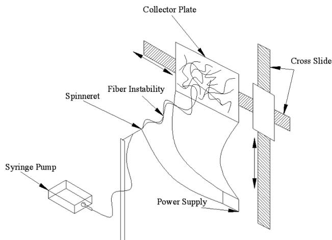
Figure (5) : Schematic for Electrospinning [10].
