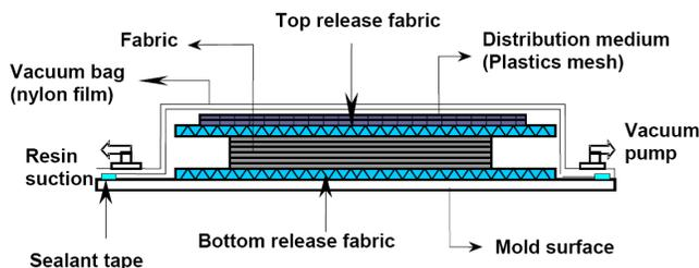
Figure (2) : VARTM setup at BVUCOE, Pune.
