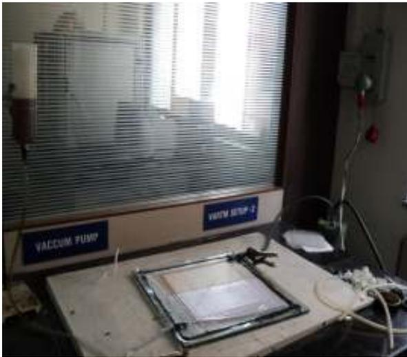
Figure (1) : VARTM processing instrument.
