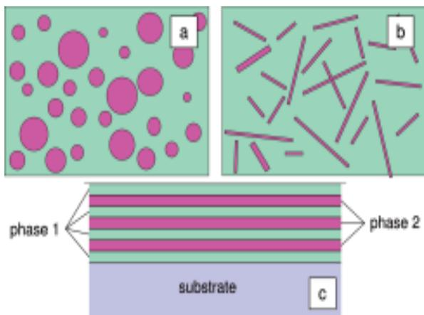
Figure (4) : Three basic types of nanocomposite. (a) Composite consisting of zero-dimensional particles in a matrix; ideally, the individual particles do not touch each other. (b) One-dimensional nanocomposite consisting of nanotubes or nanorods distributed in a second matrix. (c) Two-dimensional nanocomposite built from stacks of thin films made of two or more different materials (Source 25)
