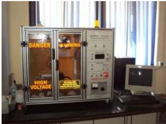
Figure (6) : Actual Setup for Electrospinning Process at BVUCOE, Pune
