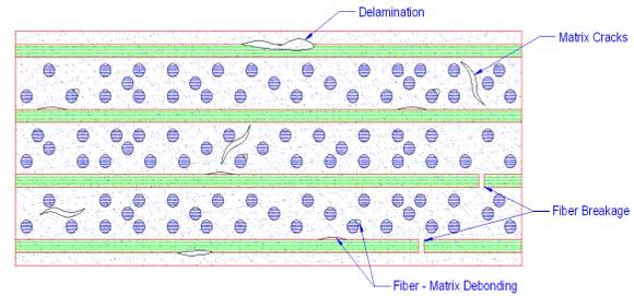
Figure (3) : Various Failure Modes in Composites
