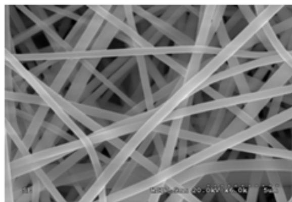
Figure (9) : Setup 3: 18 kV and 70 mm: 515 nm average fiber diameter.
