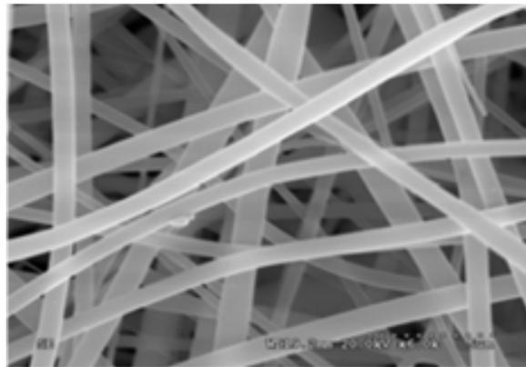
Figure (8) : Setup 2: 15 kV and 100mm. 740 nm average fiber diameter.
