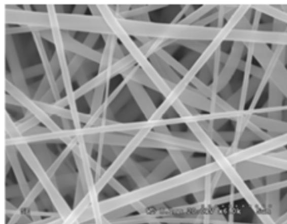
Figure (10) : Setup 4: 18 kV and 100 mm: 665 nm average fiber diameter.
