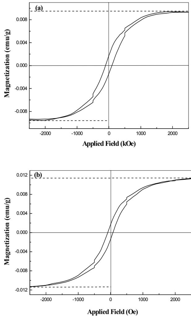
Figure (4) : Room temperature magnetic hysteresis loop of Ni<sub>0.01</sub>Zn<sub>0.99</sub>O nanoparticles calcined at (a) 400 °C and (b) 500 °C for 2 h in ambient air.
