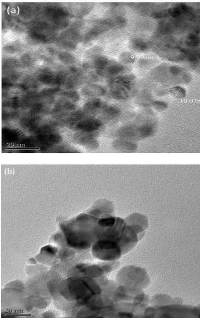
Figure (3) : TEM micrographs of (a) pristine ZnO and (b) Ni<sub>0.05</sub>Zn<sub>0.95</sub>O nanoparticles calcined at 400 °C for 2 h in ambient air.
