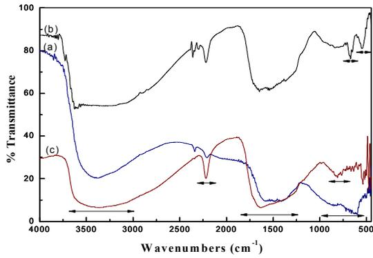
Figure (2) : FTIR spectra of (a) pristine ZnO, (b) Ni<sub>0.01</sub>Zn<sub>0.99</sub>O, and (c) Ni<sub>0.05</sub>Zn<sub>0.95</sub>O samples calcined at 400°C for 2 h in ambient air.
