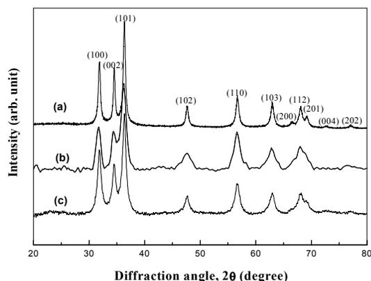
Figure (1) : X-ray diffraction in (a) ZnO nanoparticles after heating a  $\text{Zn}^{2+}$ -PVA-sucrose precursor powder at  $400^\circ\text{C}$  for 2 h, and (b)  $\text{Ni}_{0.01}\text{Zn}_{0.99}\text{O}$  and (c)  $\text{Ni}_{0.05}\text{Zn}_{0.95}\text{O}$  nanoparticles after heating the respective  $\text{Zn}^{2+}$ - $\text{Ni}^{2+}$ -PVA-sucrose precursor powders at  $400^\circ\text{C}$  for 2 h in ambient air.
