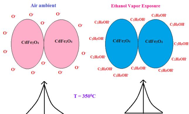
Figure (5) : Gas sensing mechanism of  $\text{CdFe}_2\text{O}_4$  at  $350^\circ\text{C}$ .
