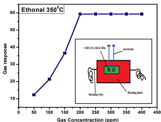
Figure (4) : Response characteristics of the  $\text{CdFe}_2\text{O}_4$  film to ethanol at  $350^\circ\text{C}$ . The right insert shows a schematic image of sensor structure.
