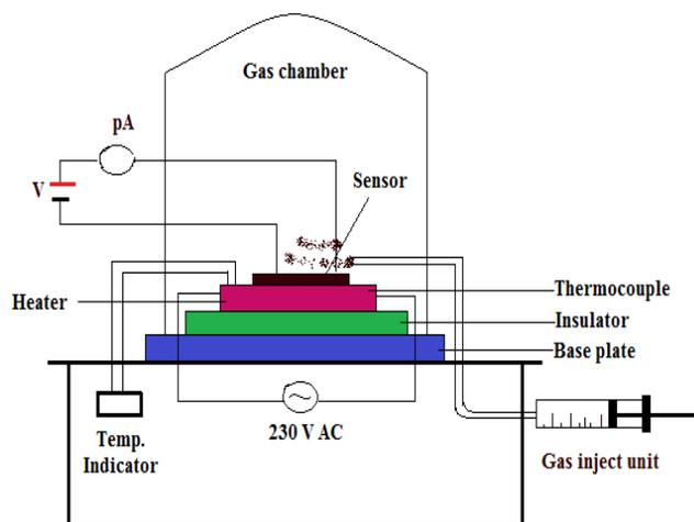
Figure (1) : Block diagram of static gas sensing setup.
