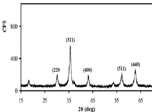
Figure (2) : X-ray diffraction patterns of CdFe $_2$ O $_4$  as synthesized Powder
