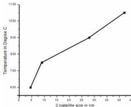
Figure (4) : Crystallite Size vs Temperature graph of Nanopowders
