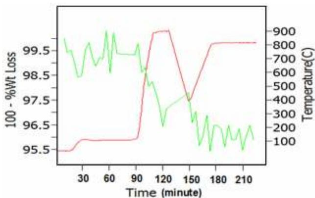
Figure (2) : Graph showing the weight loss of sample with respect to increment in temperature.
