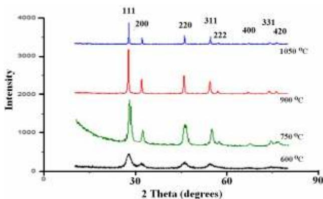
Figure (3) : XRD pattern for Naopowder Calcined at 600°C, 750°C, 900°C and 1050°C.
