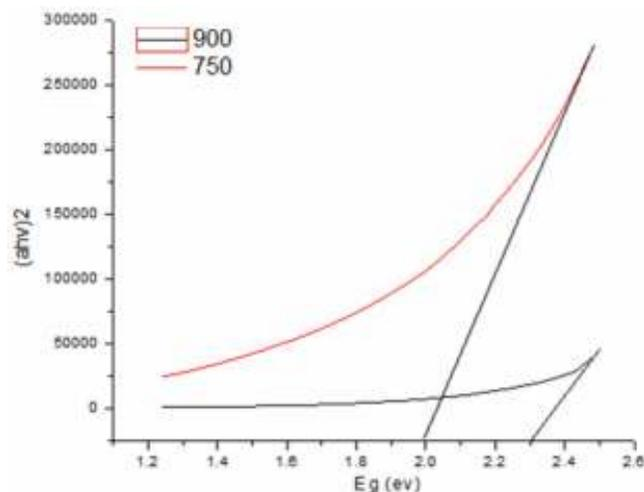
Figure (9) : Plot of  $(\alpha hv)^2$  vs  $hv$  for 750°C and 900°C.
