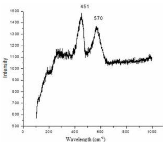
Figure (8) : Laser Raman Spectroscopic graph of Nanopowder Calcined at  $900^\circ\text{C}$ .
