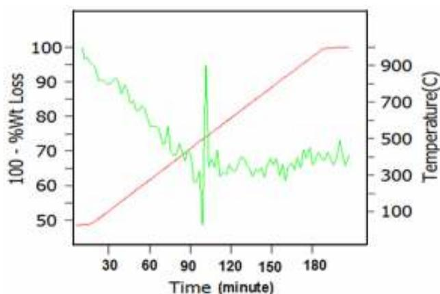
Figure (1) : Graph showing the weight loss of sample with respect to increment in temperature
