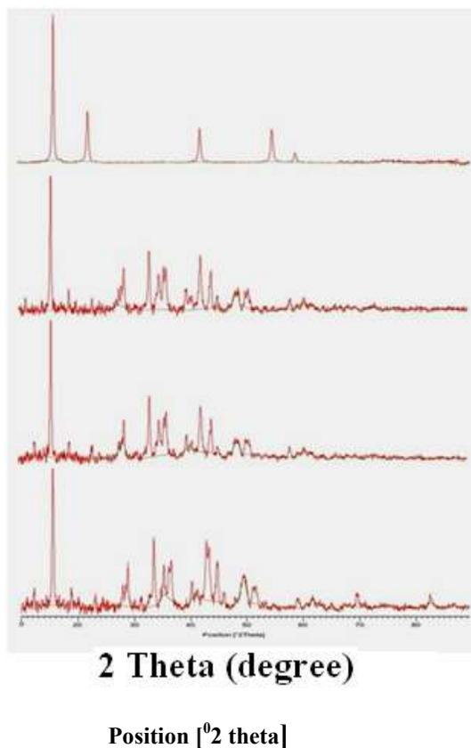
Figure (2) : XRD spectrum of silver nanoparticles (a) uncapped Ag, (b) CD (5 mM) capped Ag, (c) CD (10 mM) capped Ag and (d) CD (15 mM) capped Ag.
