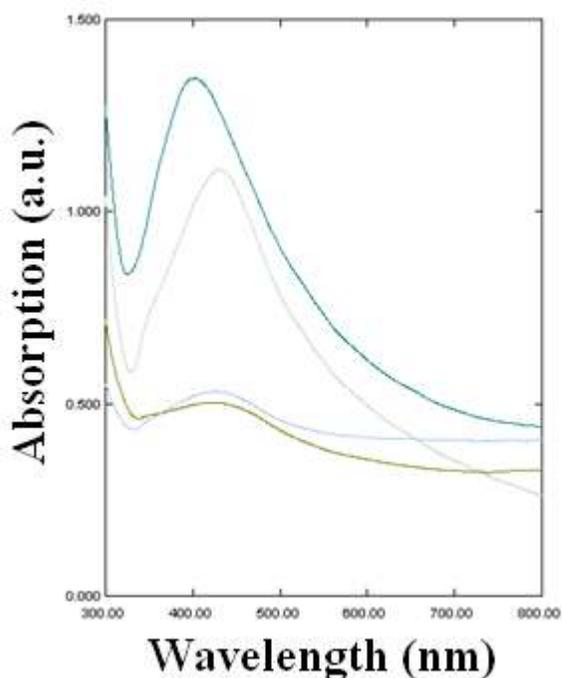
Figure (1) : UV-Visible spectrum of silver nanoparticles a) 425 nm for uncapped Ag, b) 420 nm for CD (5 mM) capped Ag, c) 414 nm for CD (10 mM) capped Ag and d) 402 nm for CD (15 mM) capped Ag.
