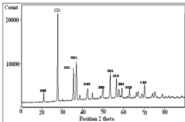
Figure (3) : X-ray diffraction pattern of  $\text{CuGeO}_3$
