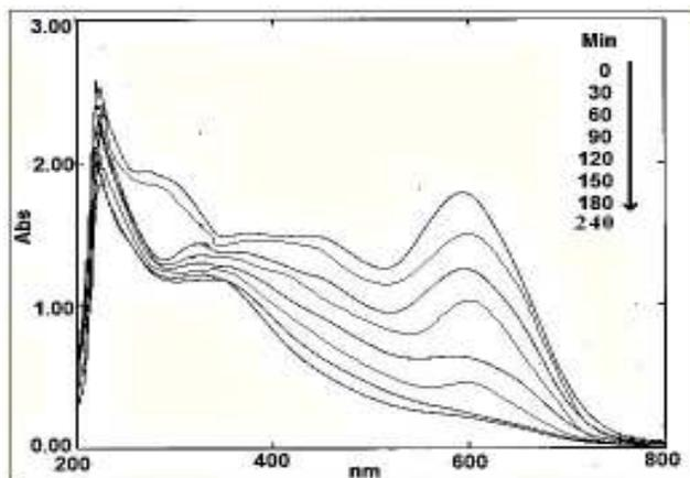
Figure (6) : UV-visible spectra of degraded dye
