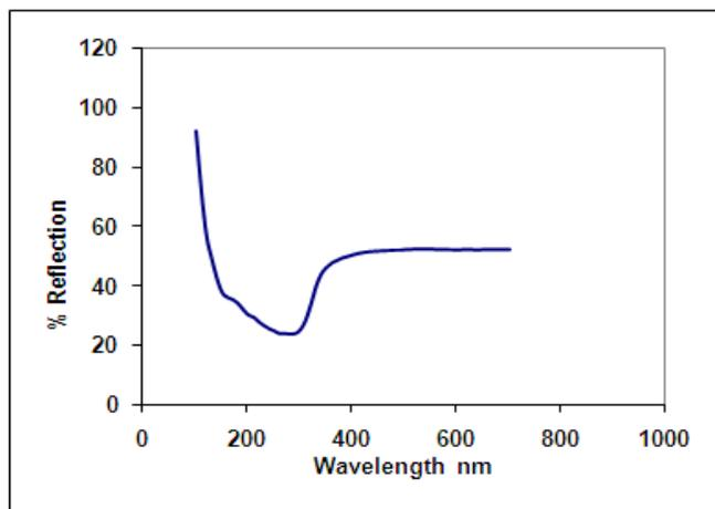
Figure (2) : UV-visible spectra of  $\text{CuGeO}_3$
