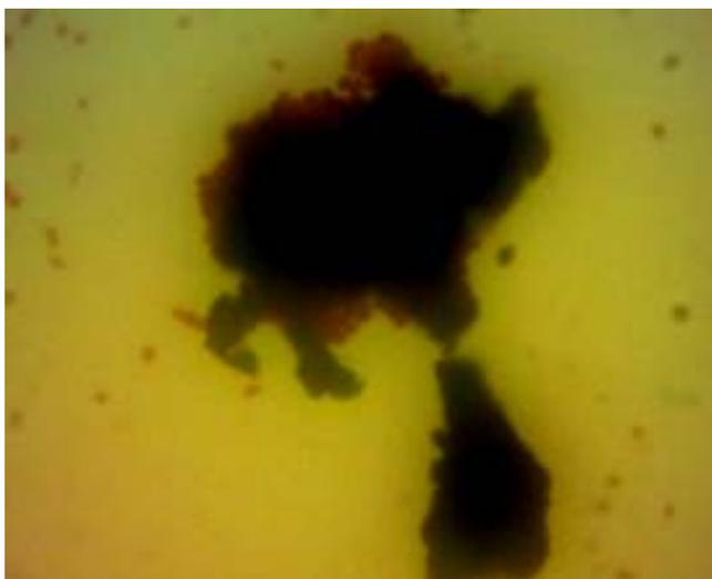
Figure (7) : *E. Coli* absorbed on Graphite aggregates.
