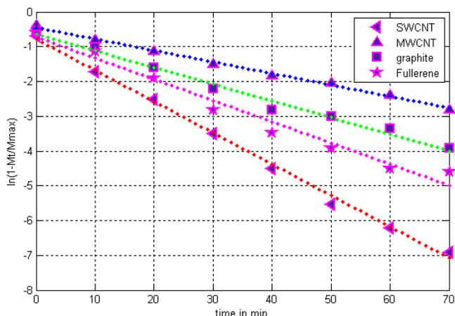
Figure (2) : Correlation of adsorption kinetics data with diffusion model for *E.coli* on different nano carbon aggregates at 25°C
