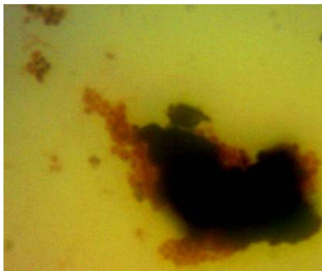
Figure (5) : *E.coli* adsorbed on Fullerene aggregates.
