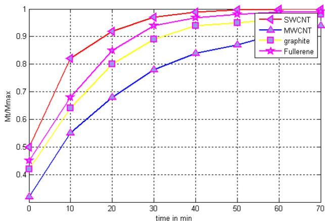
Figure (1) ; Fractional uptake curve of *E.coli* on SWCNT, MWCNT, graphite, fullerene Aggregates.
