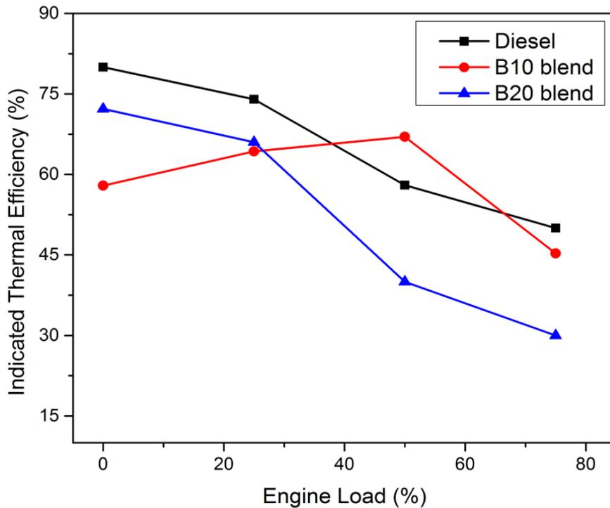
Figure (2): Variation of indicated thermal efficiency at different engine loads.
