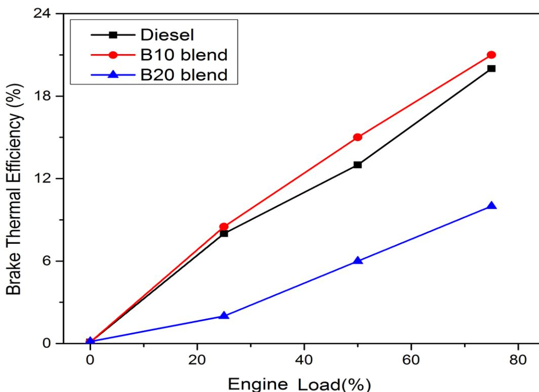
Figure (1): Variation of brake thermal efficiency at different engine loads.
