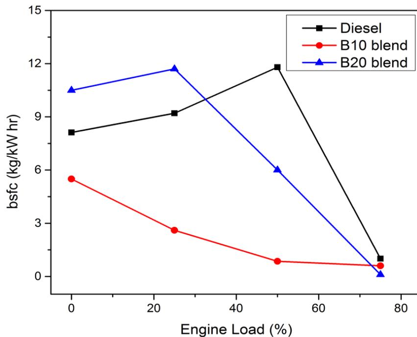
Figure (3): Variation of brake specific fuel consumption at different engine loads.
