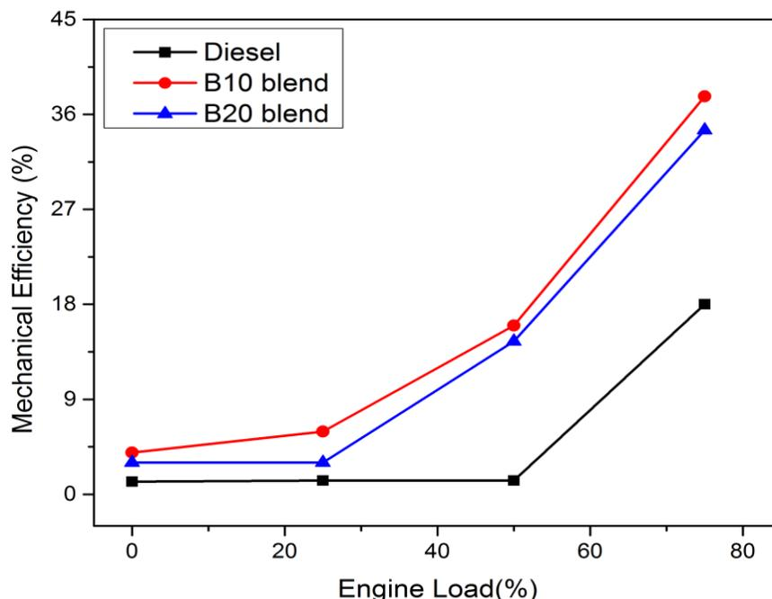
Figure (4): Variation of mechanical efficiency at different engine loads.
