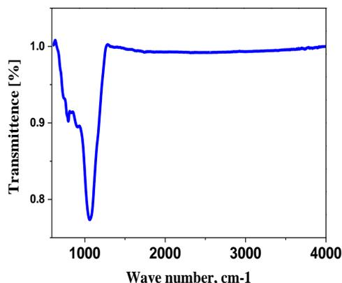
Figure (2): FTIR spectra of raw fly ash powder
