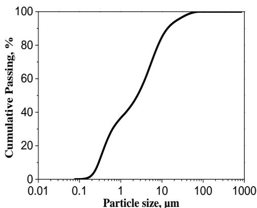
Figure (1): Particle size distribution of raw fly ash powder
