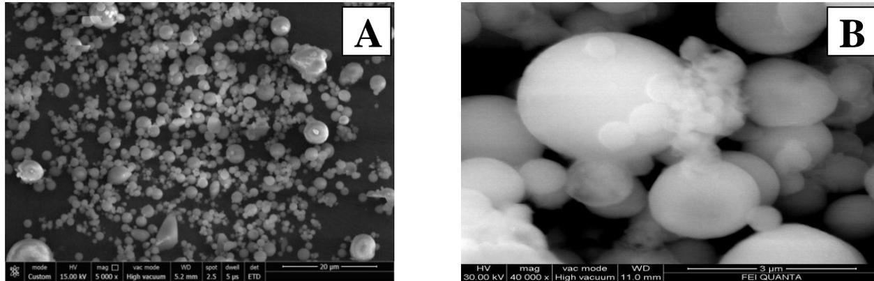
Figure (3): Morphology of raw fly ash powder
