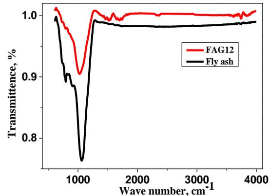
Figure (5): FTIR spectra of FAG12 geopolymer sample
