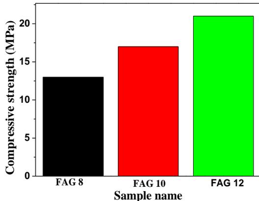
Figure (4): Compressive strength under artificial curing
