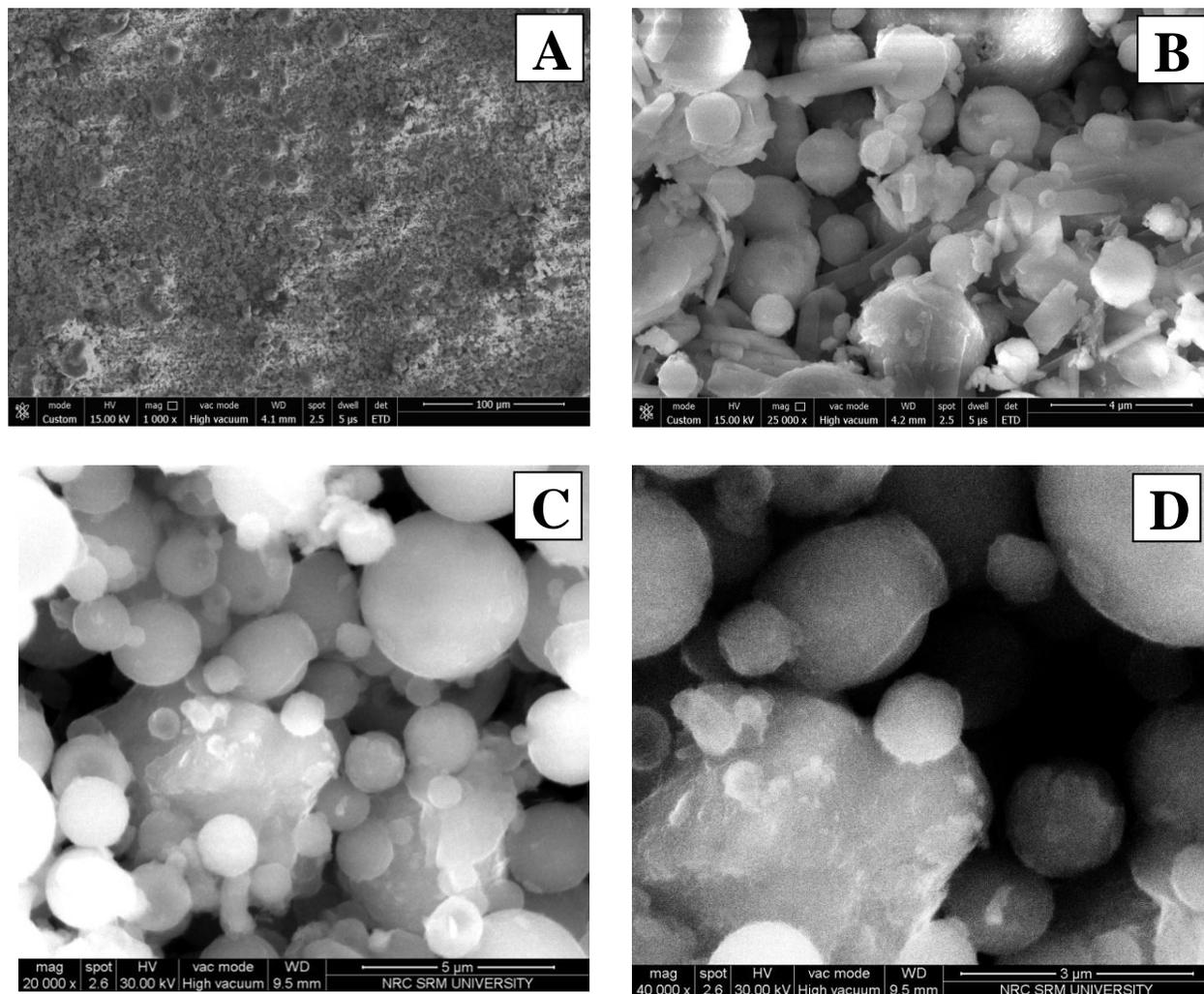
Figure (6): SEM micrographs of FAG12 geopolymer sample cured at 60 °C
