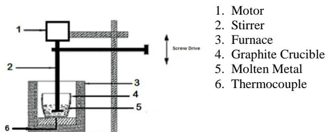
Figure (3): Experimental set up by stir casting route.
