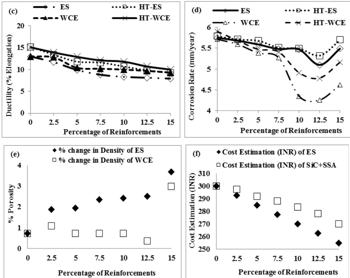
Figure (4): Tribo-mechanical properties of hybrid green AMC.
