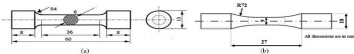
Figure (2): (a) Tensile and (b) fatigue sample.
