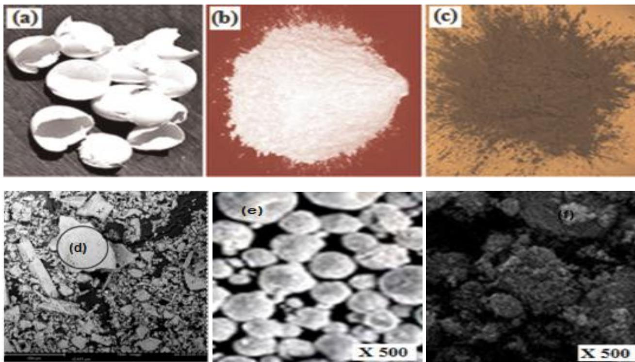
Figure (1): Pictures of (a) eggshells, (b) ES powder, (c) WCE powder, (d) SEM morphology of SiC+SSA, (e) SEM morphology of ES, (f) SEM morphology of WCE.
