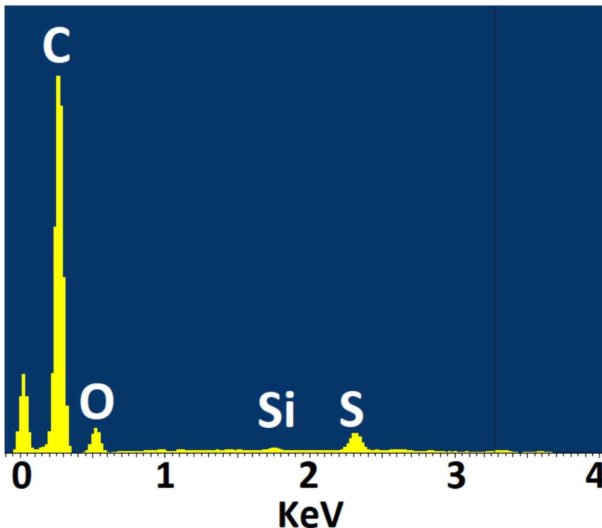
Figure (5). Elemental composition analysis by EDX spectra for glassy carbon mould material.
