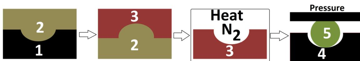
Figure (1). Schematic flowchart for aspherical glass lens fabrication using glassy carbon mould. Indications: Tungsten carbide master mould (1); PDMS replication (2); Phenolic mixture (3); Cured resin after carbonization process (4) and Glass precursor (5).
