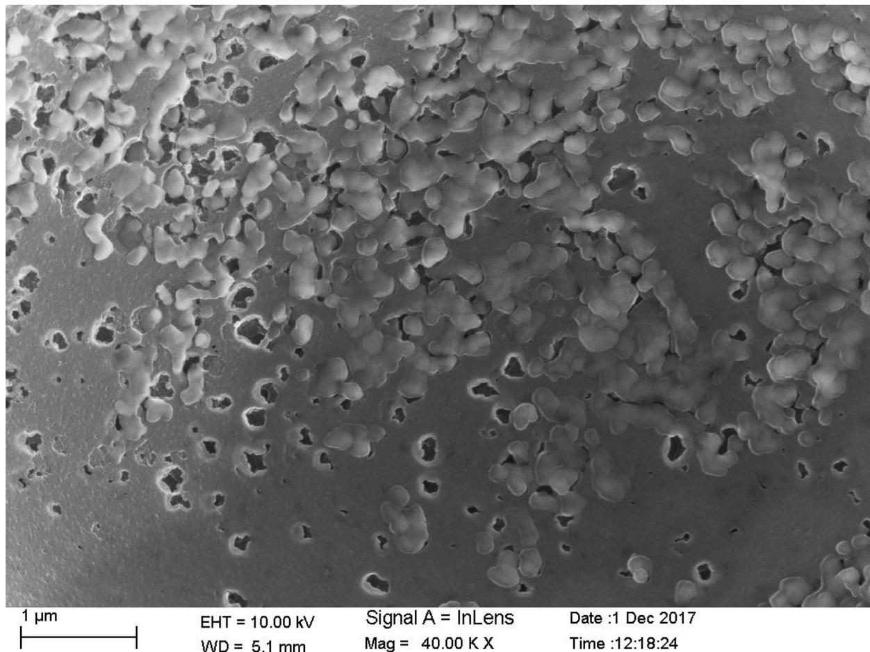
Figure (4). Microstructure and surface quality analysis by FESEM of glassy carbon mould material.
