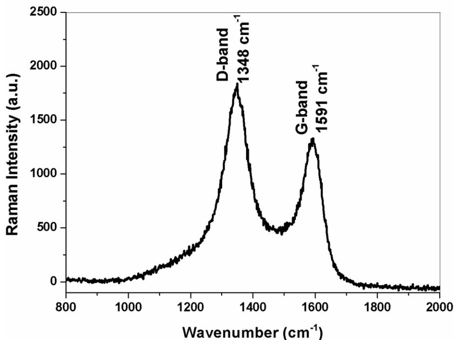
Figure (3). Raman spectra of fabricated glassy carbon mould.
