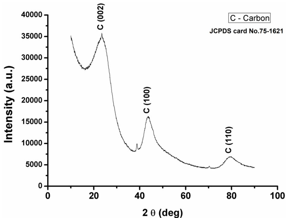
Figure (2). XRD pattern of fabricated glassy carbon mould.
