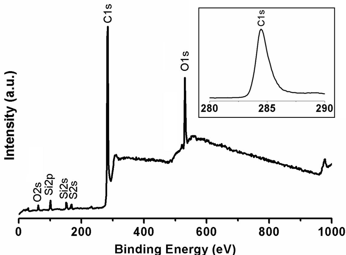
Figure (6). XPS analysis of glassy carbon mould material.
