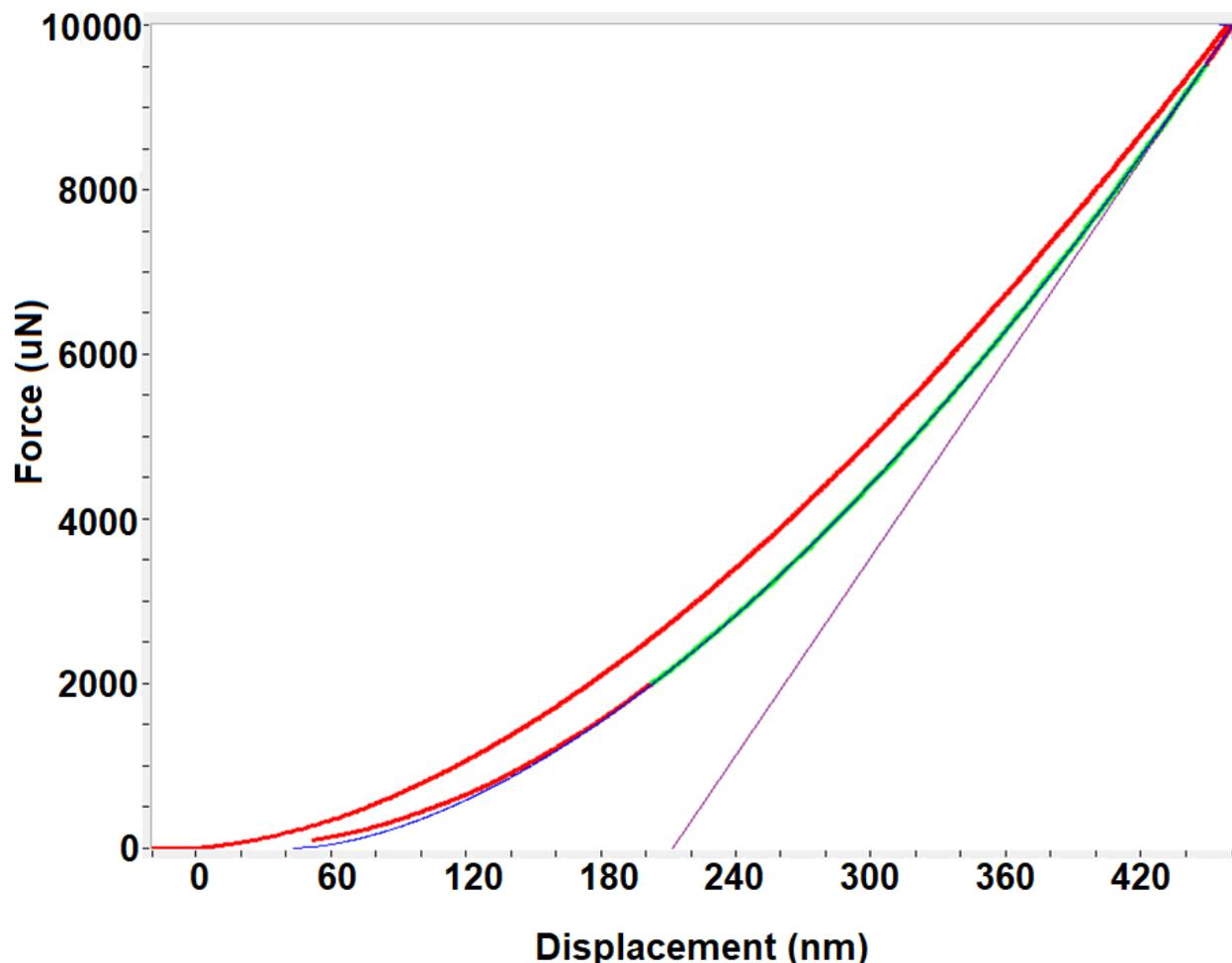
Figure (7). Hardness testing fabricated glassy carbon block by nanoindentation.
