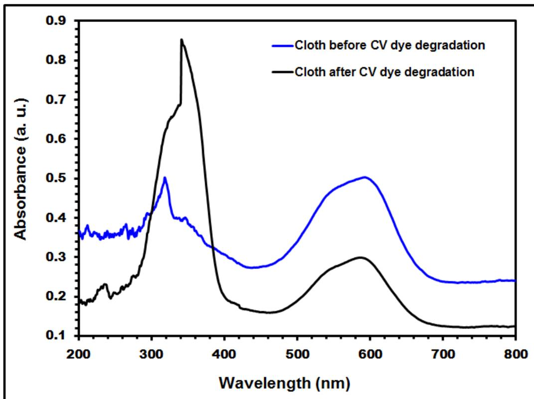
Figure (2): UV-VIS spectra of the cloth before and after photocatalytic washing.
