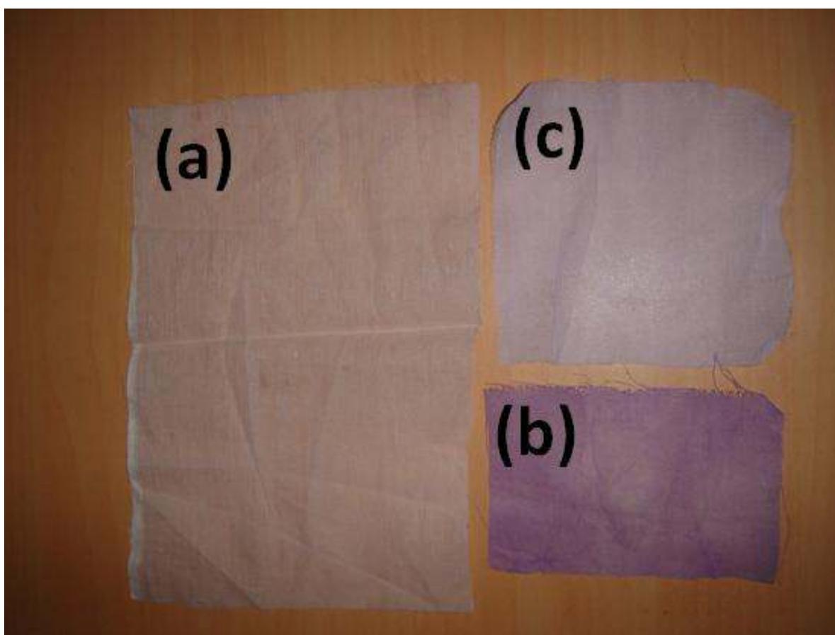
Figure (1). Photograph of the white color cotton cloth used in the process (a); CV stained cotton cloth (b); and photocatalytically washed cotton cloth (c).
