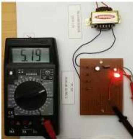
Figure (1.12): 5V DC Power Supply.
