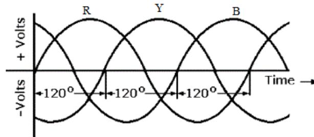
Figure (1.1): Three Phase System Waveform [8].
