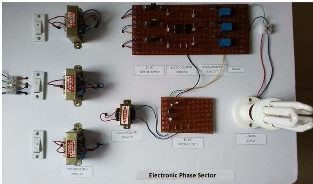
Figure (1.11): Hardware Model of the Electronic Phase Selector Switch.
