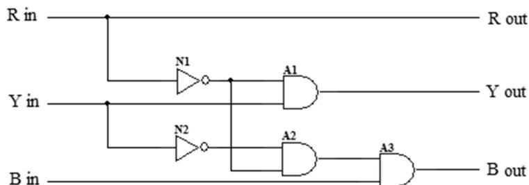
Figure (1.4): Logic Control Circuit
