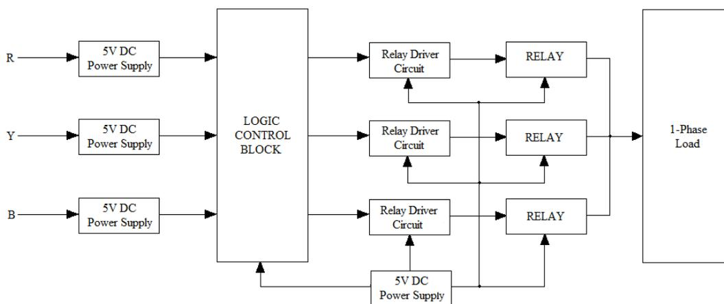
Figure (1.2): Block Diagram of Electronic Phase Selector Switch.
