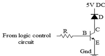
Figure (1.9): Relay Driver Circuit [9].
