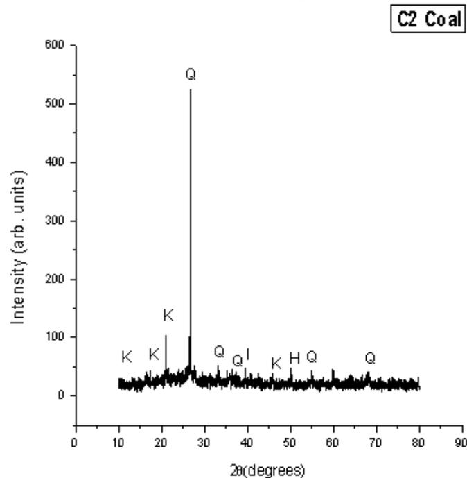
Figure (1): XRD patterns of raw coal. Q-quartz; K-kaolinite I-illite, H: hematite.
