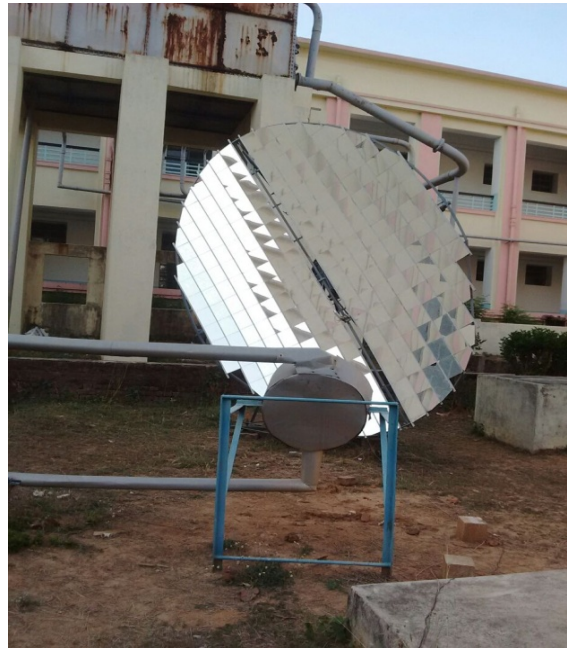
Figure (1): Experimental setup of Scheffler concentrator placed in BIT Mesra, Ranchi.
