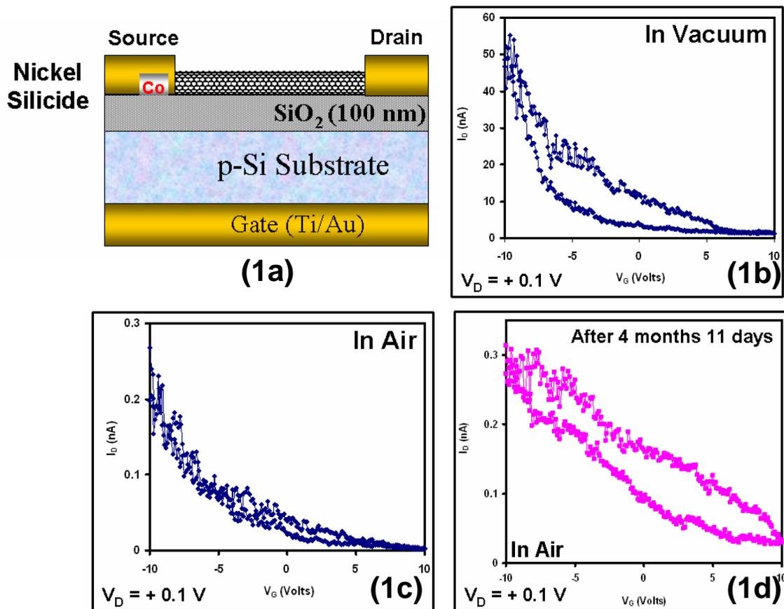
Figure (1): (a) Schematic of the back gate SWCN FET with nickel silicide as source and drain electrodes, (b)  $I_D$ - $V_G$  characteristic of the SWCN FET in Vacuum after annealing - showing p-type FET, (c)  $I_D$ - $V_G$  characteristic of the SWCN FET measured just after breaking vacuum (i.e. in ambient air atmosphere). (d)  $I_D$ - $V_G$  characteristic of the SWCN FET measured in air after 4 months and 11 days.
