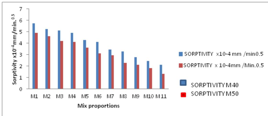
Figure (8): Sorptivity values for M40 and M50 grade concrete.
