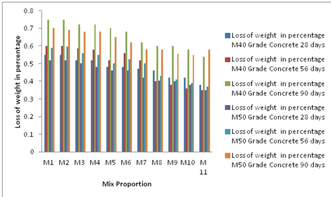
Figure (10): Alkaline Resistance for M40 and M50 Grade of Concrete.
