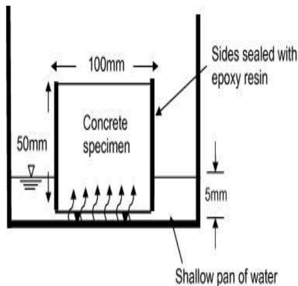
Figure (3): Sorptivity test set up.
