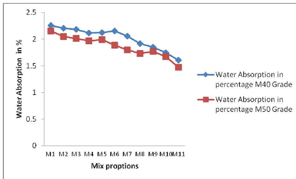
Figure (6): Water absorption test for M40 and M50 grade concrete.
