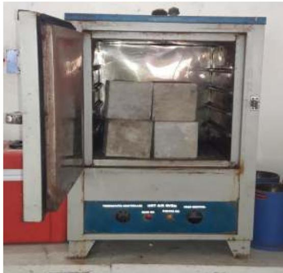
Figure (1): Experimental setup of the water absorption test.
