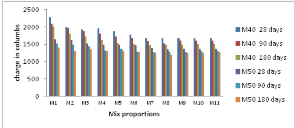
Figure (7): RCPT values for M40 and M50 grade concrete.
