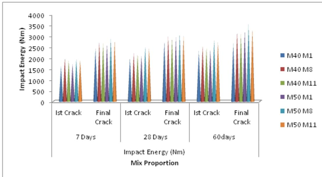
Figure (11): Impact resistance of the concrete of grade M40 and M50.
