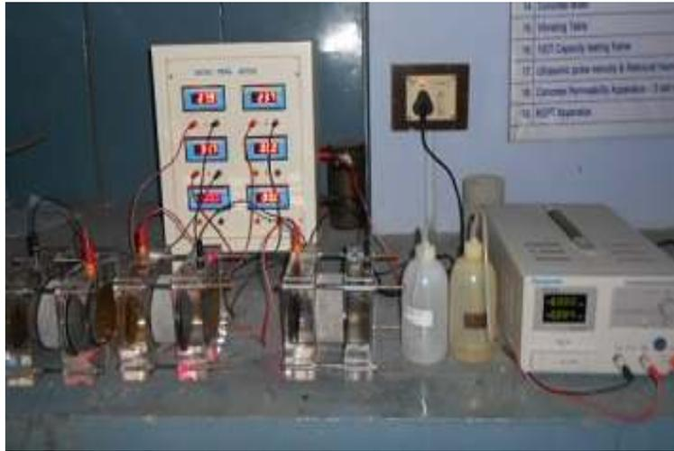
Figure (2): Rapid chloride permeability test setup.
