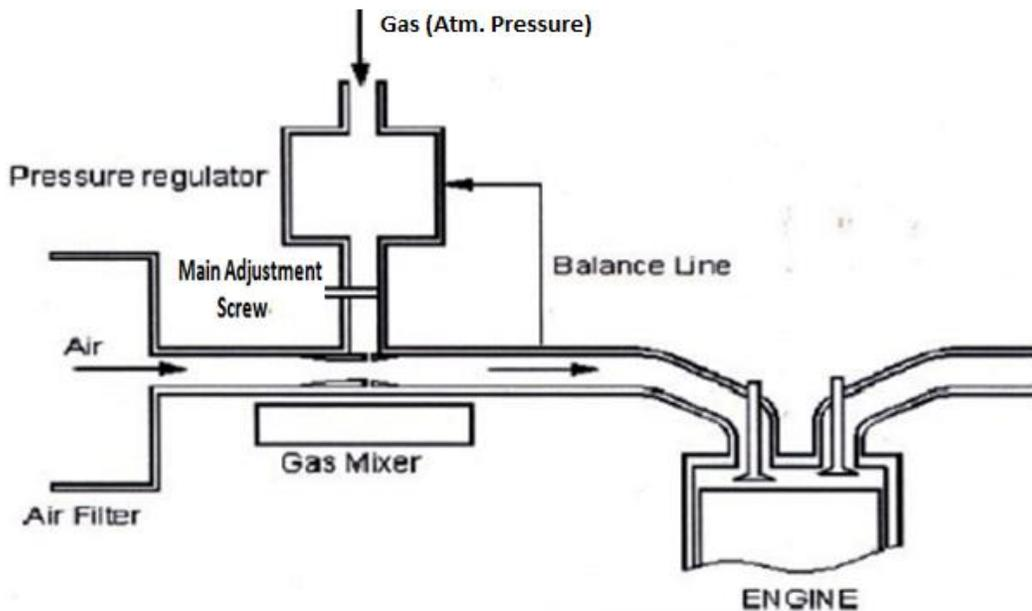
Fig 3: Schematic Diagram of Air, Gas and Mixture Flow
