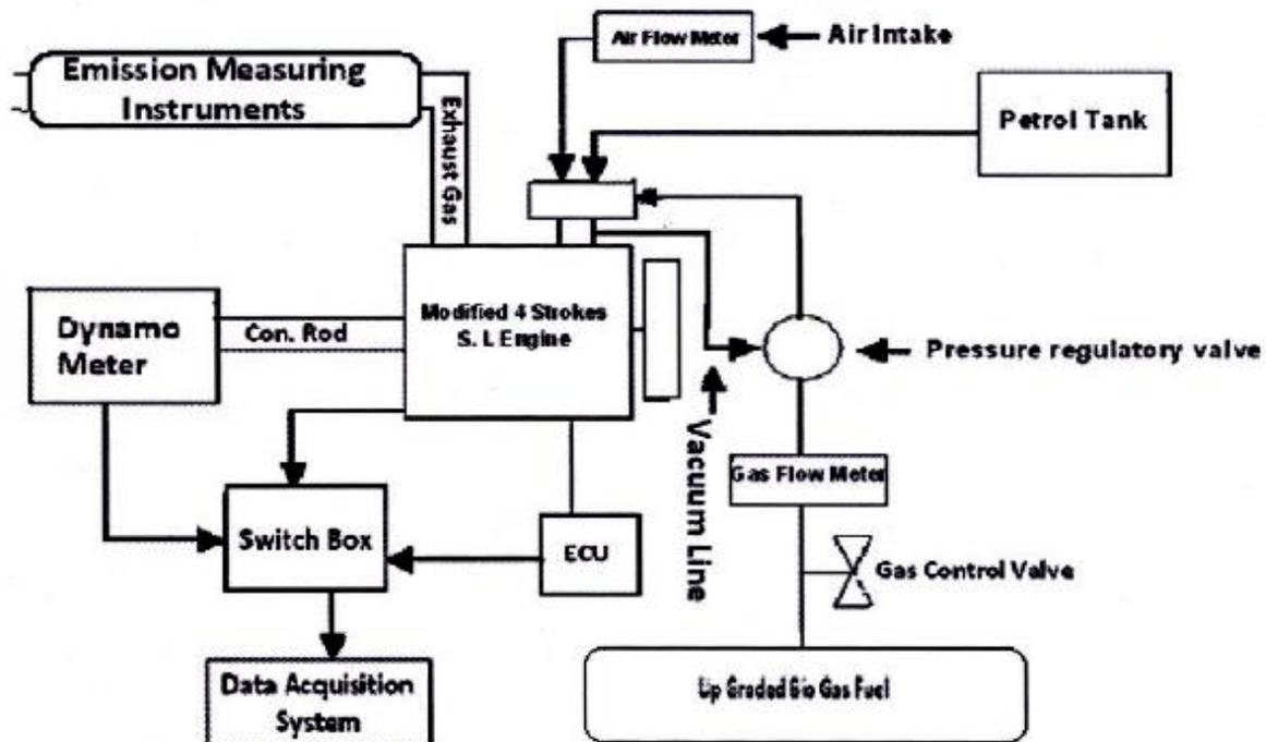
Figure 4: Experimental Set-up of Modified 4 Stroke S. I. Engine.
