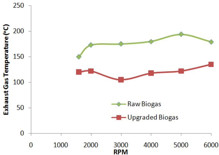
Figure 9: Exhaust Gas Temperature v/s RPM.
