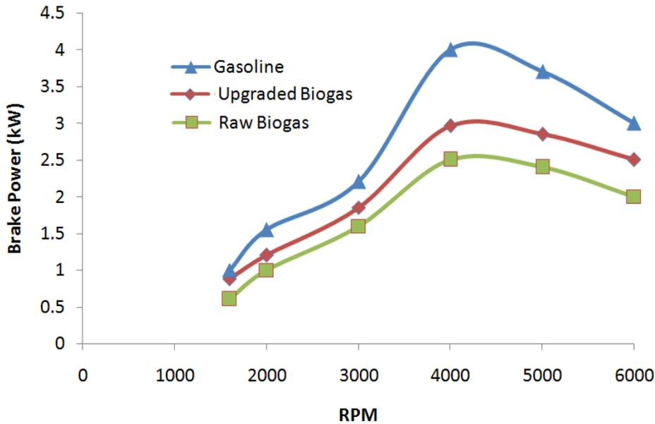
Figure 7: Engine Brake Power v/s RPM.
