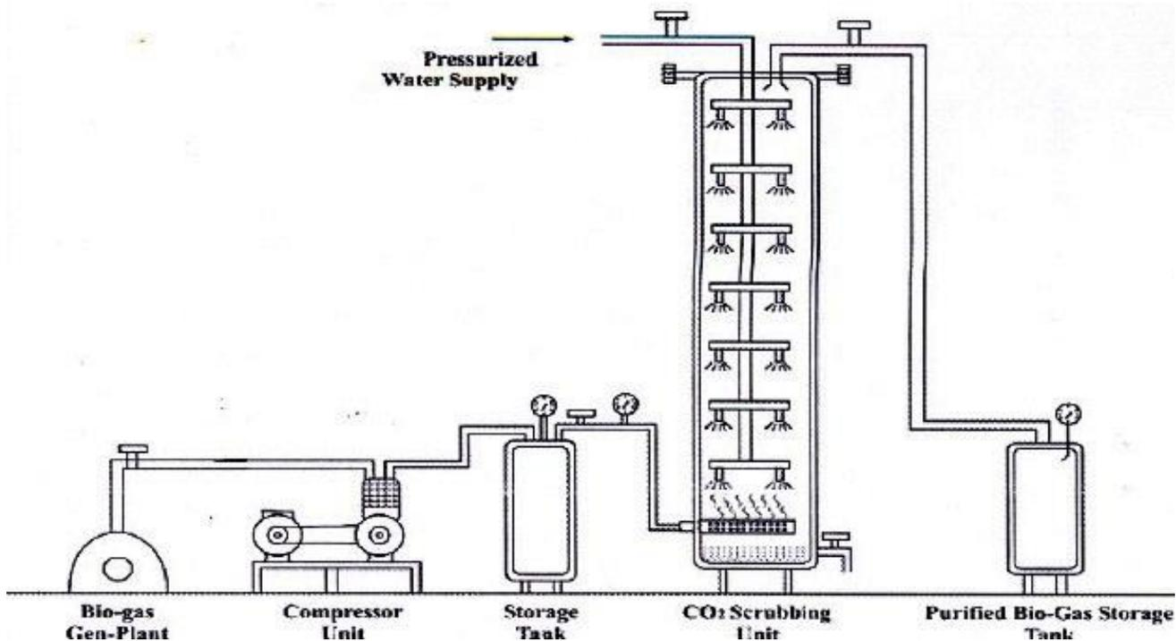
Figure 1: Biogas purification unit.
