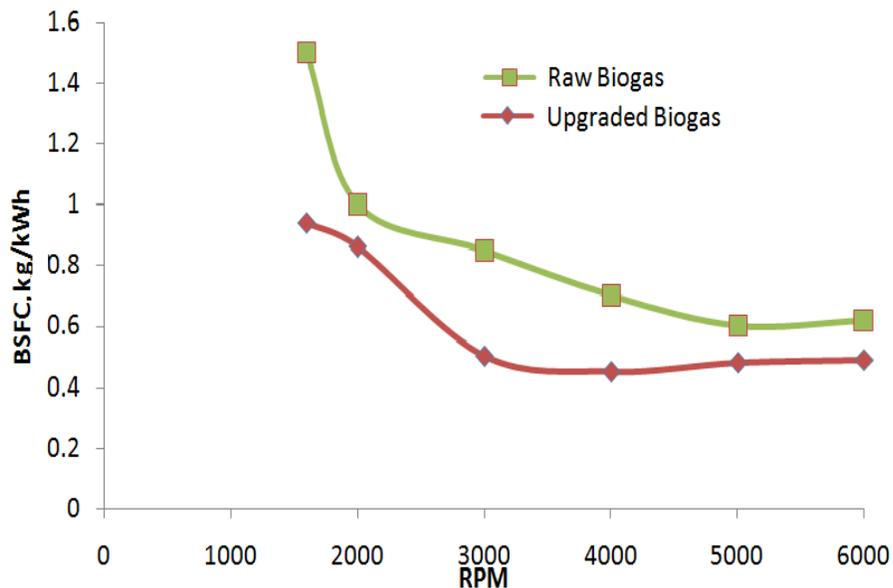
Figure 8: BSFC v/s RPM.
