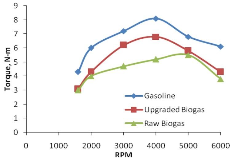
Figure 6: Engine Torque v/s RPM.
