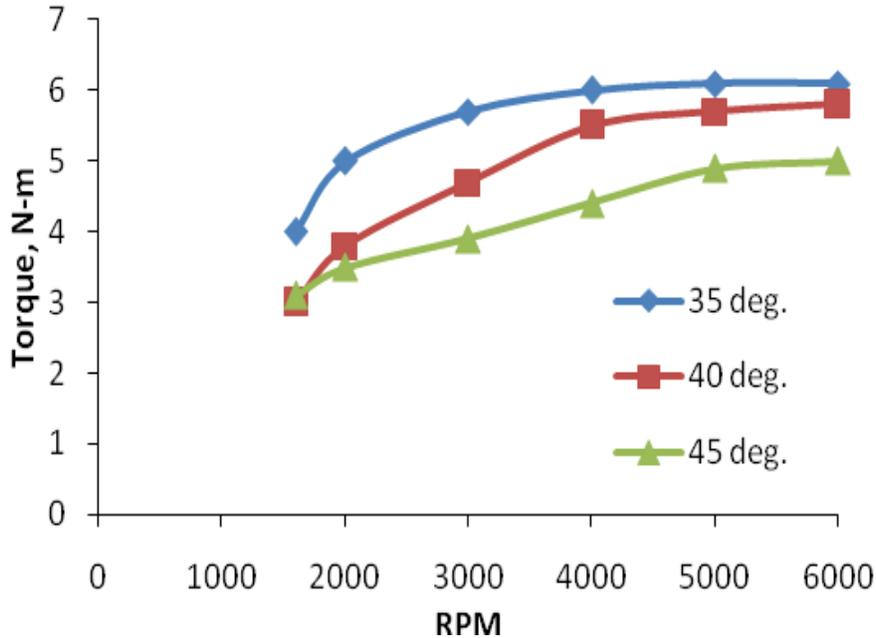
Figure 5: Biogas Fueled Engine Torque v/s Spark Advance.
