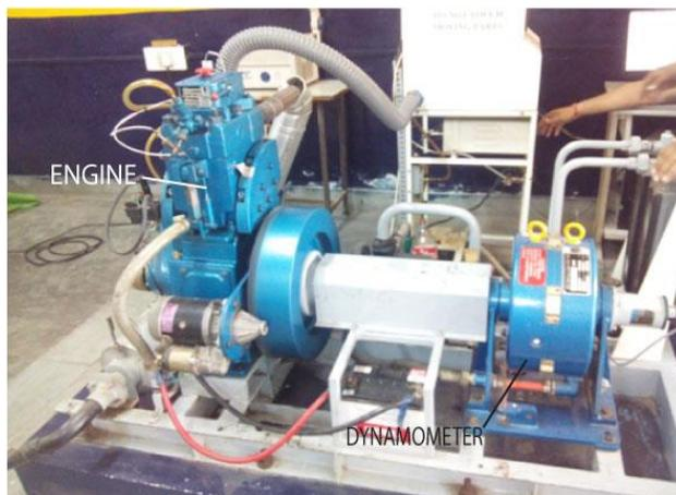
Figure 1: Variable compression research engine.
