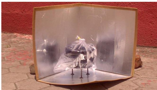
Figure (2): Reflective panel type solar cooker with two boxes.
