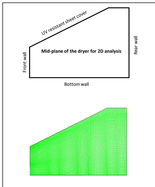
Figure (3): (a) Mid-plane of the dryer for 2D analysis and (b) meshed domain.
