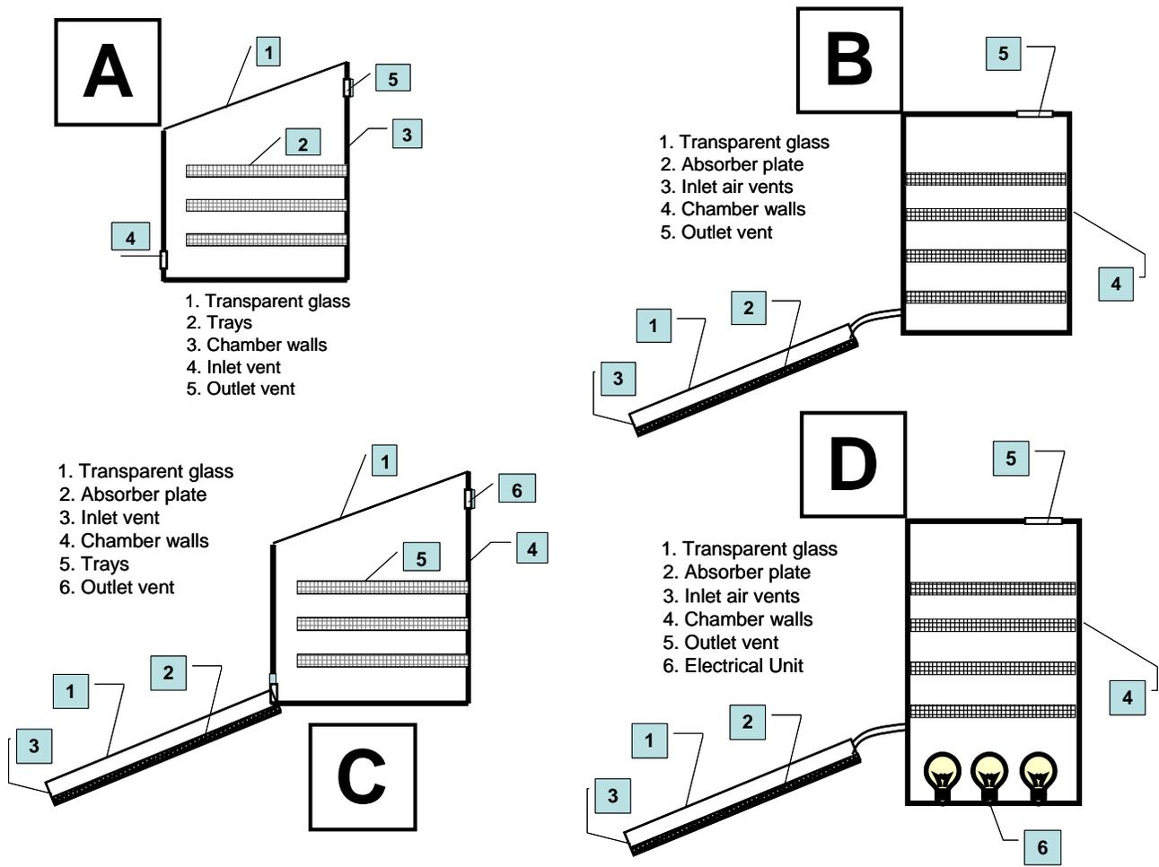
Figure (1): Schematic of (a) Direct solar dryer (b) Indirect solar dryer (c) Mixed solar dryer and (d) Hybrid solar dryer.
