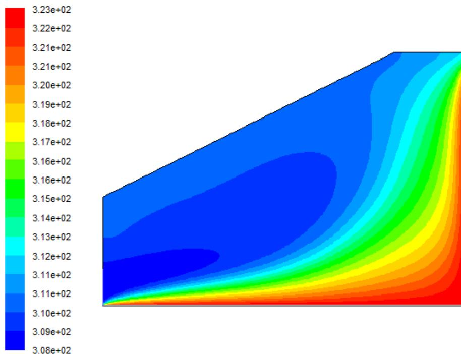
Figure (4): . Temperature distribution for LOC-FR configuration of the dryer.
