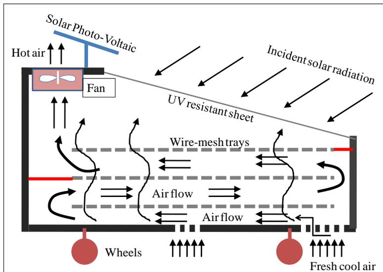
Figure (2): Schematic of forced convection direct solar dryer.
