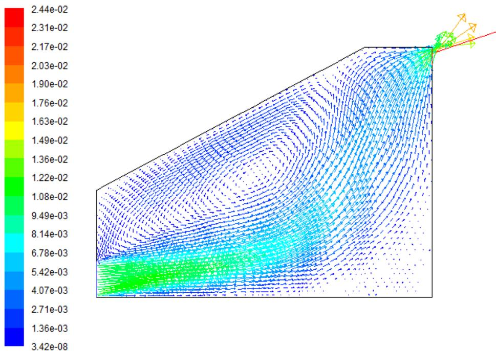
Figure (6): . Veolcity vectors for LOC-FR configuration of the dryer.
