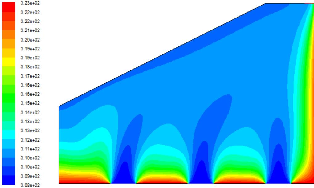
Figure (7): . Temperature distribution for LOC-BT configuration of the dryer.
