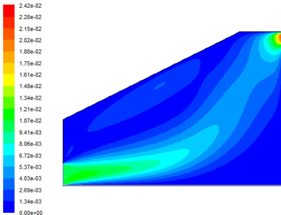
Figure (5): . Air velocity distribution for LOC-FR configuration of the dryer.
