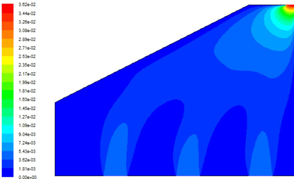
Figure (8): . Air flow distribution for LOC-BT configuration of the dryer.
