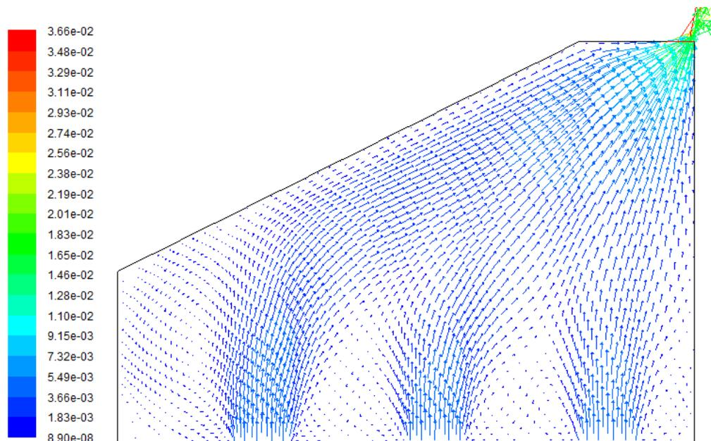
Figure (9): . Velocity vectors for LOC-BT configuration of the dryer.
