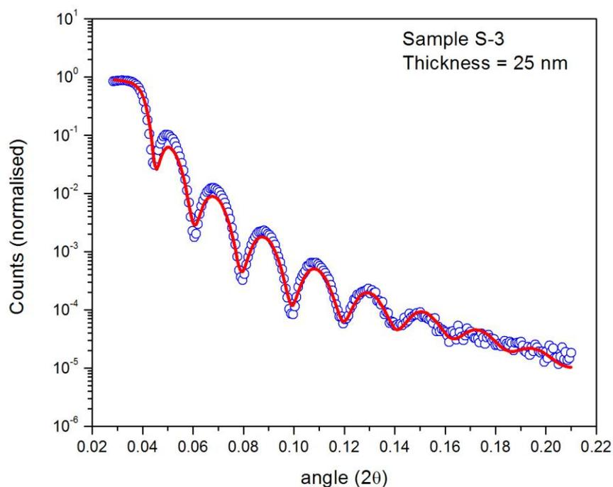
Figure (2): Calculation of thin film thickness by using XRR of sample S-3.
