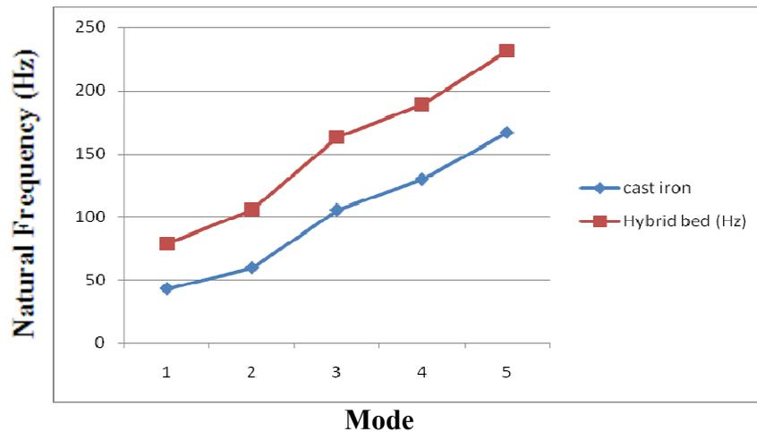
Figure (6): Natural frequencies of cast iron bed and Hybrid bed
