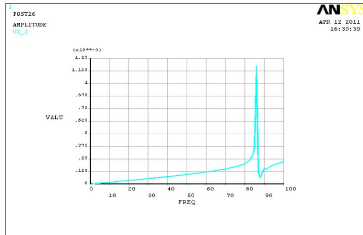
Figure (10): Displacement vs frequency for hybrid bed under harmonic loading conditions
