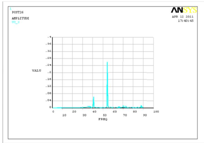
Figure (9): Displacement vs frequency for CI bed under harmonic loading conditions
