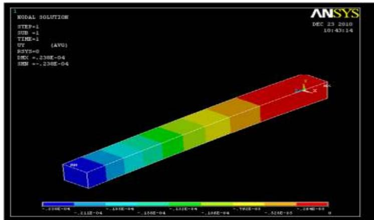
Figure (3): Deformation of 2mm plate
