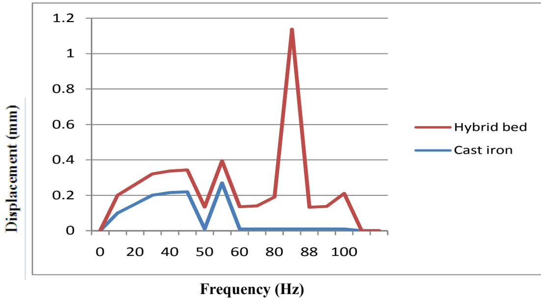
Figure (11): Harmonic analysis result of cast iron and hybrid bed
