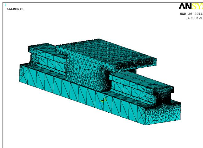
Figure (8): Meshed model of VMC bed
