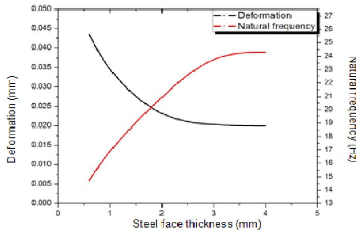
Figure (4): Steel face thickness vs deformation and natural frequency of hybrid samples of different plate thicknesses
