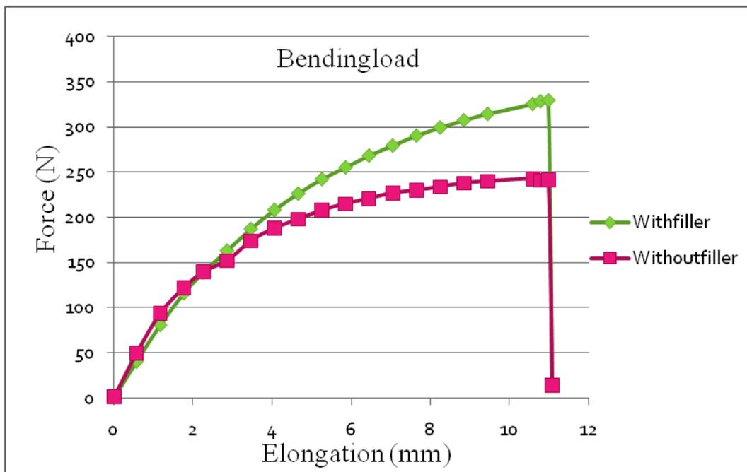
Figure (7): Variation of Flexural Load with Displacement for the Composites with and Without Fillers.
