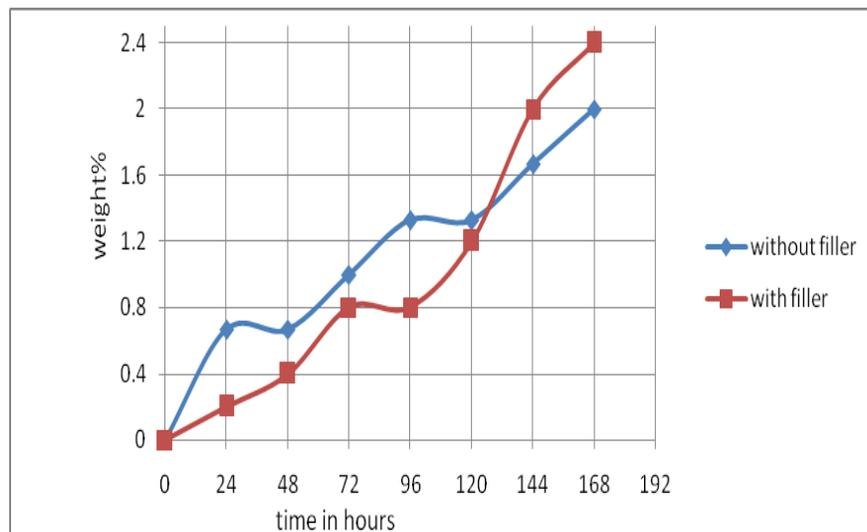
Figure (9): Variation of Water Absorption of the Composites With Respect To Time.
