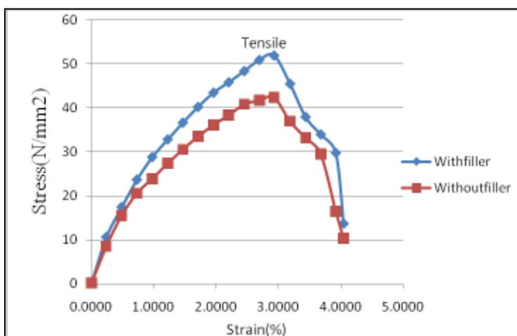
Figure (5): Variation of Tensile Stress with Strain for Composite with Fillers and Without Fillers.
