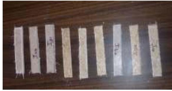
Figure (3): Impact test specimen of various laminates.
