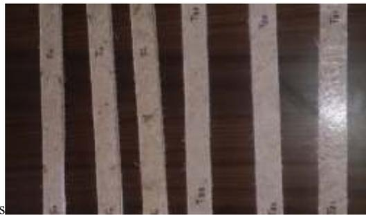
Figure (1): Tensile test specimen of various laminates
