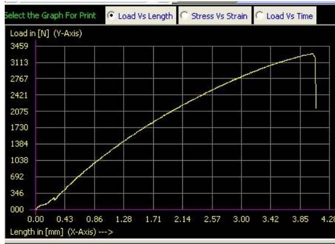
Figure (4): Load Vs deflection curve (GSGBG)
