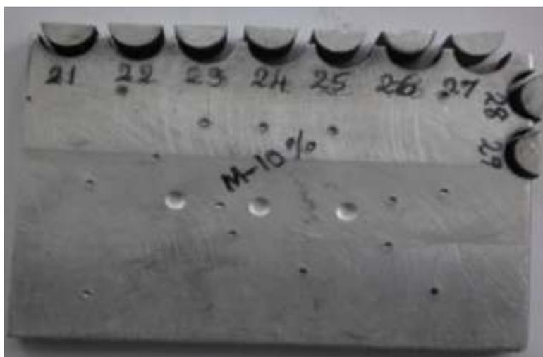
Figure (8): The machined AA6063/10%SiC plate.
