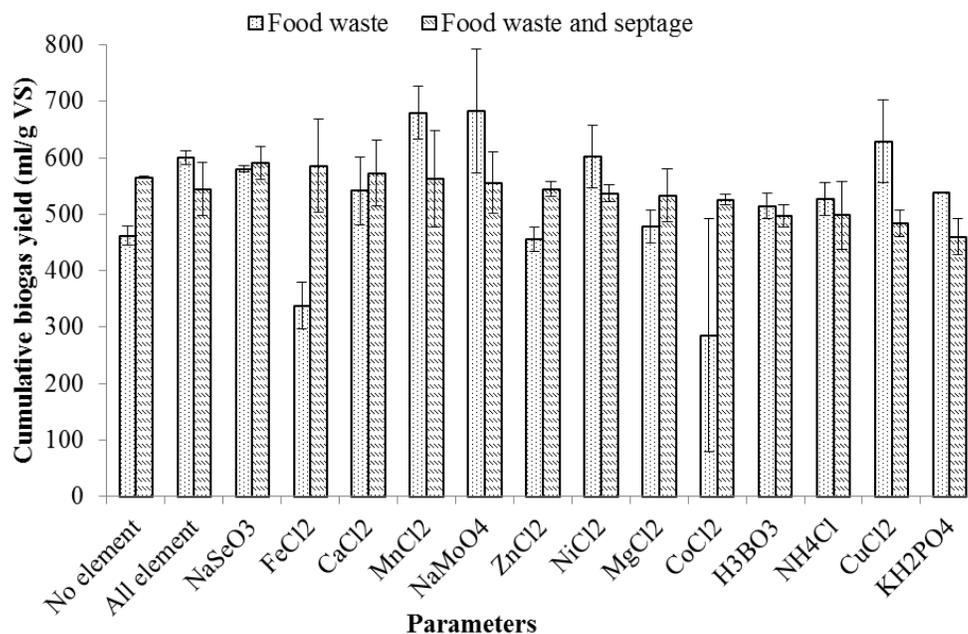
Figure (4): The cumulative production in ml/g VS of biogas from FW and mixture of FW and septage with nutrient limiting condition. The results show that co-digestion of FW and septage with proper mixing ratio can improve biogas production probably supplementing trace elements.
