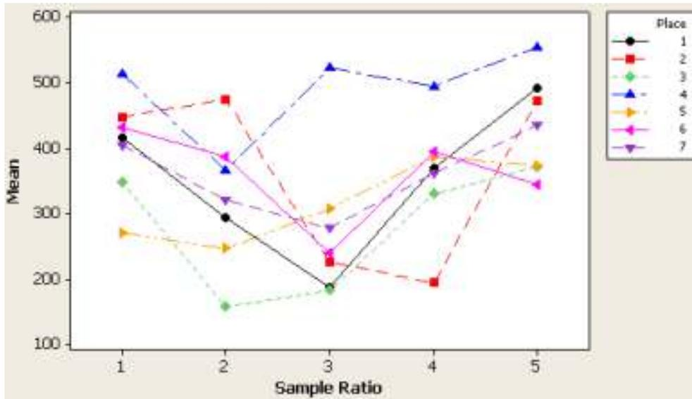
Figure (2): 2-D Interaction plot of methane production for different samples. X-axis, sample mixing ratios 1, 2, 3, 4 and 5 correspond to 1:1, 1.5:1, 2:1, 1:1.5 and 1:2 respectively. Places 1, 2, 3, 4, 5, 6 and 7 correspond to Panchavati, Nashik East (NE), Nashik West (NW), Satpur, CIDCO, Nashik Road (NR) and mixed samples.
